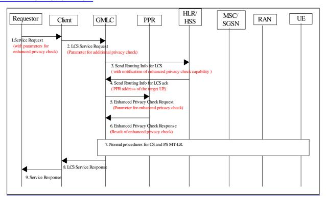
Figure 7.1.1; General information flow for the architectural alternative with the PPR attached to GMLC
