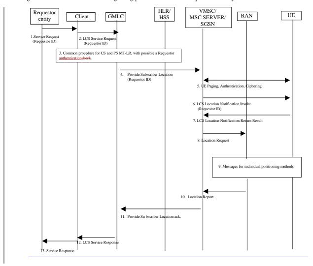
Figure 8.1; MT-LR signaling procedure when the requestor identity is authenticated in GMLC
