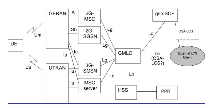
Figure 7.4; LCS architecture alternative with PPR attached to HLR
