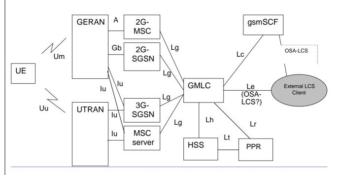
Figure 7.1; LCS architecture alternative with PPR attached to GMLC
