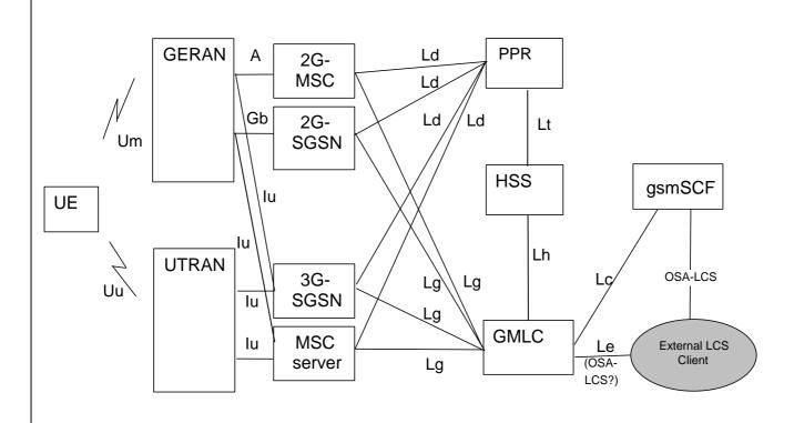
Figure 7.2; LCS architecture alternative with PPR attached to MSC/SGSN
