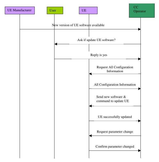
Figure 4: UE Software Update Sequence Diagram
