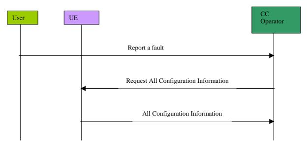
Figure 2: UE Configuration Query Sequence Diagram
