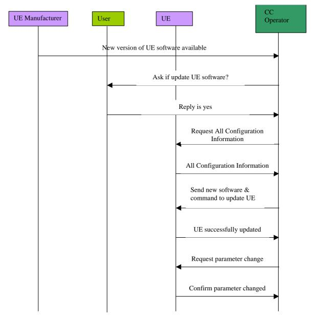
Figure 4: UE Software Update Sequence Diagram
