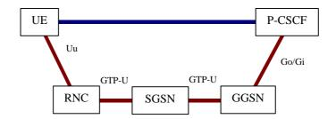
The solution to these concerns is to provide confidentiality between UE and P-CSCF at the SIP or upper IP layer (i.e. UE and P-CSCF terminate the encryption). This fits in better with the concept of the IM domain being independent of the PS domain. The encryption key Ckim, which is already negotiated during the IM authentication could be used. Since we are applying the integrity mechanism at the UE and P-CSCF, confidentiality could be applied at the same level without much more effort.
