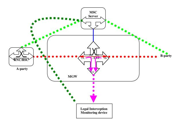
We have assumed that the encoding at the termination TLI is ITU-T G.711, and therefore we do not see the need for a new 'standard intercept control message' since the mechanisms which are already in the standard protocol over the Mc interface (ITU-T H.248) meet these requirements.
