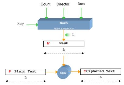
A mask M is generated that is applied to the incoming data (Plain text) P to yield the ciphered data C, according to the following equation:
