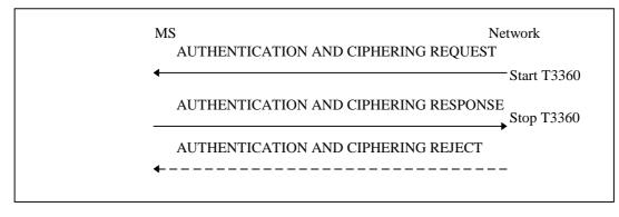
Figure 4.7.7/1 TS 24.008: Authentication and ciphering procedure
