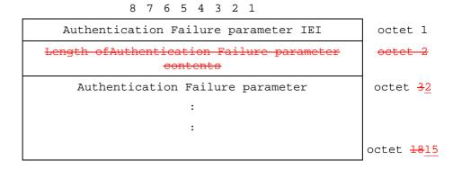
Table 10.5.90.2/TS 24.008: Authentication Failure parameter information element
