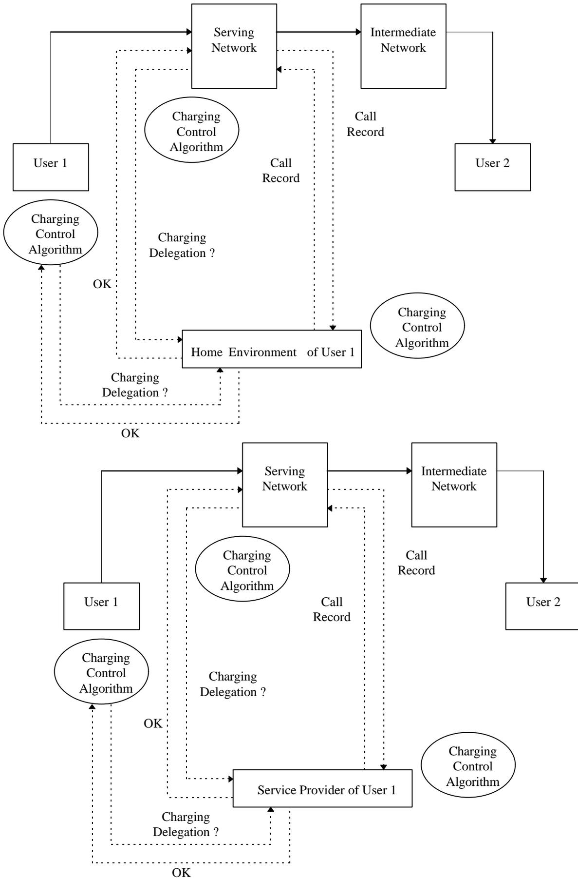
Figure 1: Charging Control Flow for Outgoing Calls
