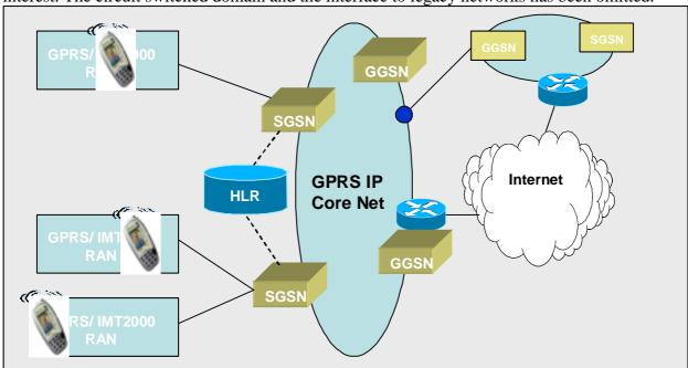
As already described in [1] TS 23.060 defines the stage 2 service description for the General Packet Radio Service (GPRS) which is a packet bearer service and a main part of the packet domain. ITU-T Recommendation I.130 describes a three-stage method for characterisation of telecommunication services
