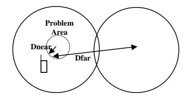
**Dnear** is the distance from the MS to the serving Node B antenna. **Dfar** is the distance from the MS to a distant Node B antenna. The near/far ratio is the ratio of **Dfar:Dnear** at which a distant Node B is a distance of Dfar from the MS and can **just** detect the signal from the MS. This ratio is a function of the propagation environment, MS transmit power and the processing gain from integration time.
