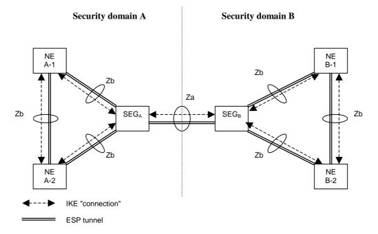
Figure 1: NDS architecture for IP-based protocols
