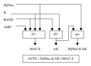
Figure 10: Construction of the parameter AUTS
