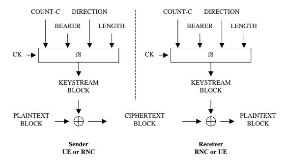
Figure 16b: Ciphering of user and signalling data transmitted over the radio access link
