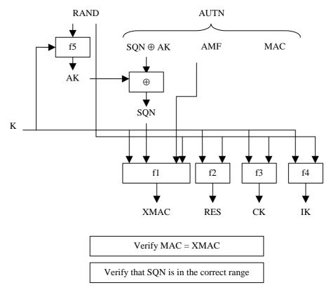
Figure 9: User authentication function in the USIM
