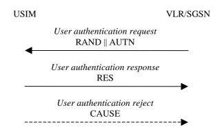
Figure 8: Authentication and key establishment
