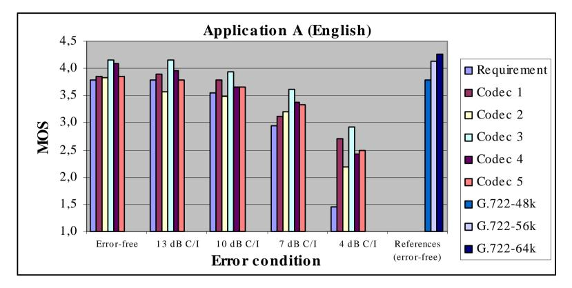
GSM FR channel with an additional constraint of 16 kbit/s A-ter sub-multiplexing (source codec < 14.4 kbit/s)
