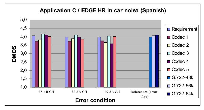
Circuit Switched EDGE/GERAN 8-PSK Phase II HR channel
