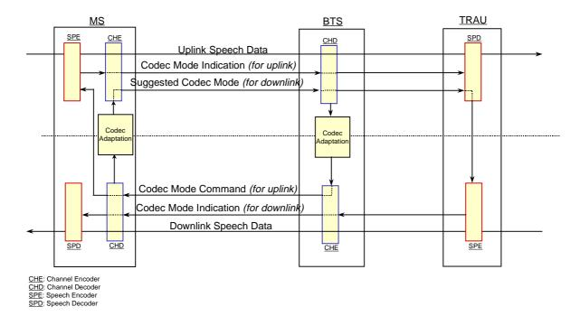
In both directions, the speech data frames are associated with a Codec Mode Indication used by the receiving end to select the correct channel and source decoders. In the network, the Codec Mode Indication must also be sent to the Transcoder Units so that the correct source decoding is selected.
