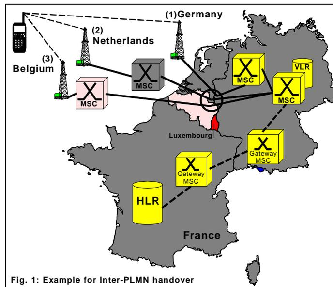
Fig. 1: Example for Inter-PLMN handover
