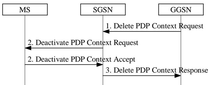
**Figure 43: PDP Context Deactivation Initiated by GGSN Procedure**
