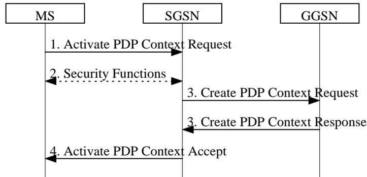
**Figure 1: PDP Context Activation Procedure**
