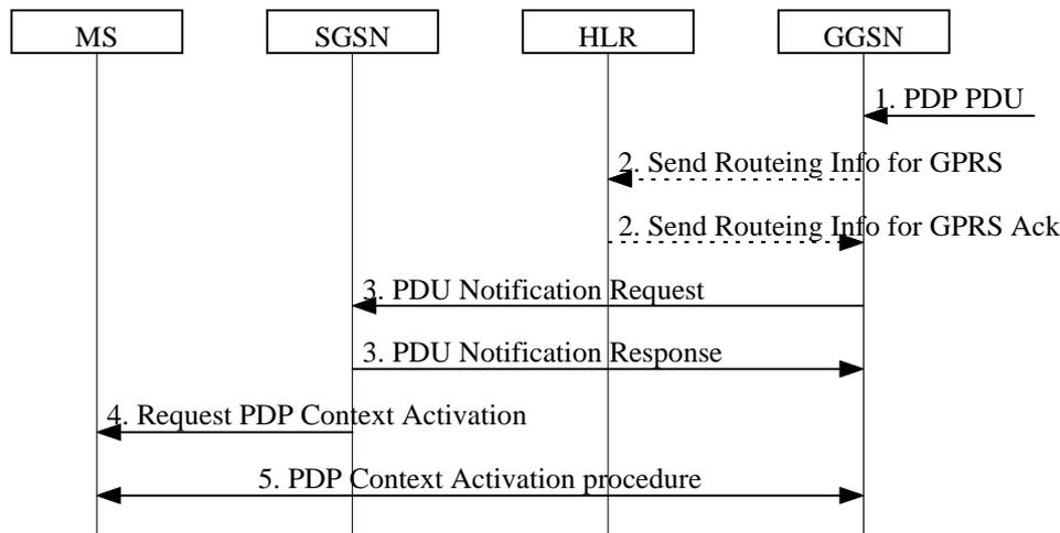
**Figure 36: Successful Network-Requested PDP Context Activation Procedure**
