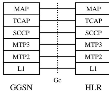
Figure 11: Signalling Plane GGSN - HLR Using MAP
