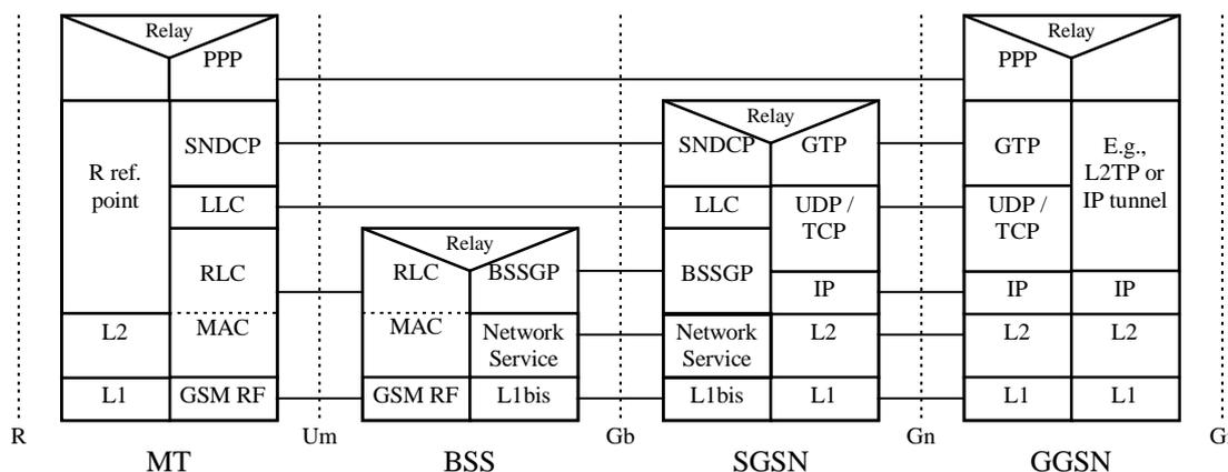
Figure 49: Transmission Plane for PDP Type PPP
