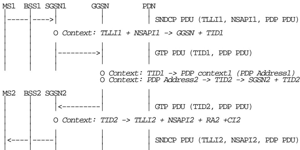
Figure C.3: MS-to-MS Data Routing via the Same GGSN
