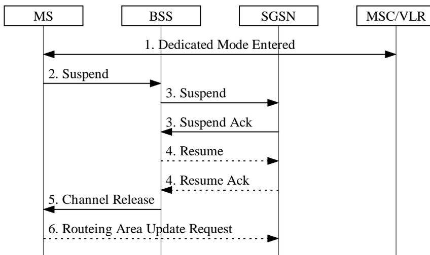
**Figure 58: Suspend and Resume Procedure**
