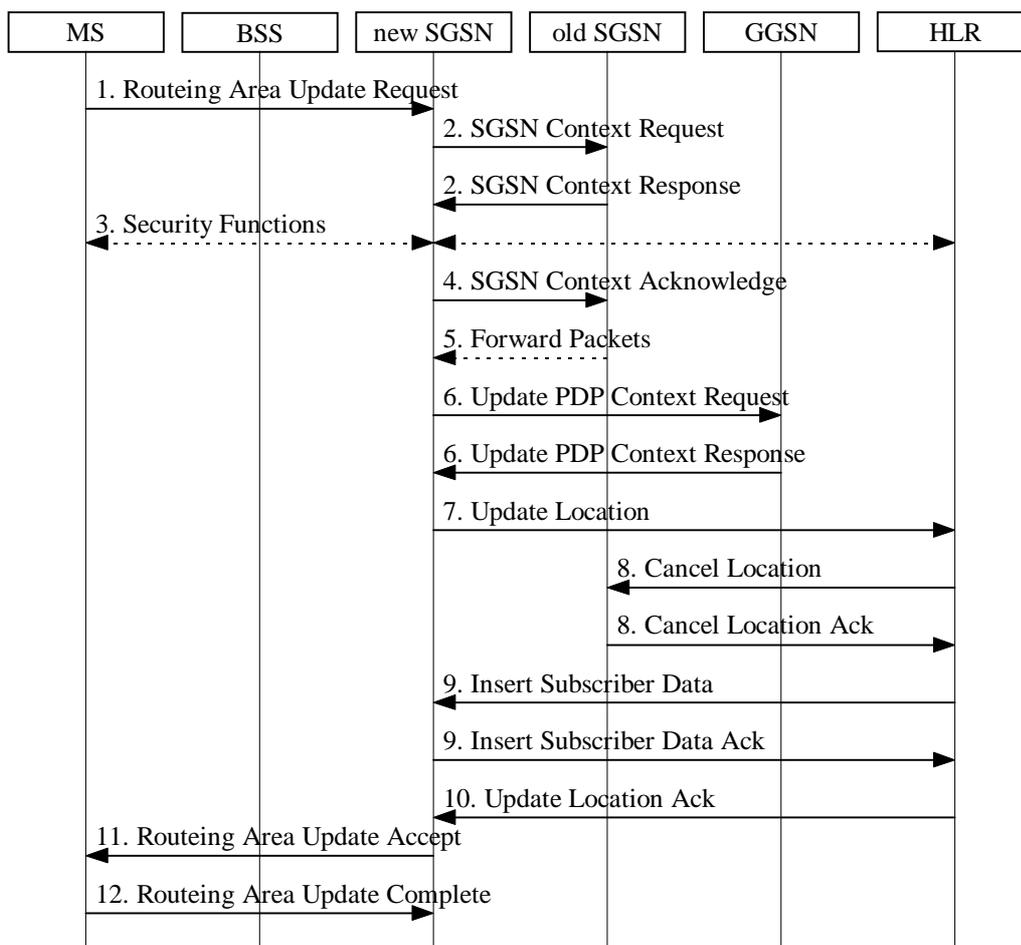
**Figure 28: Inter SGSN Routeing Area Update Procedure**
