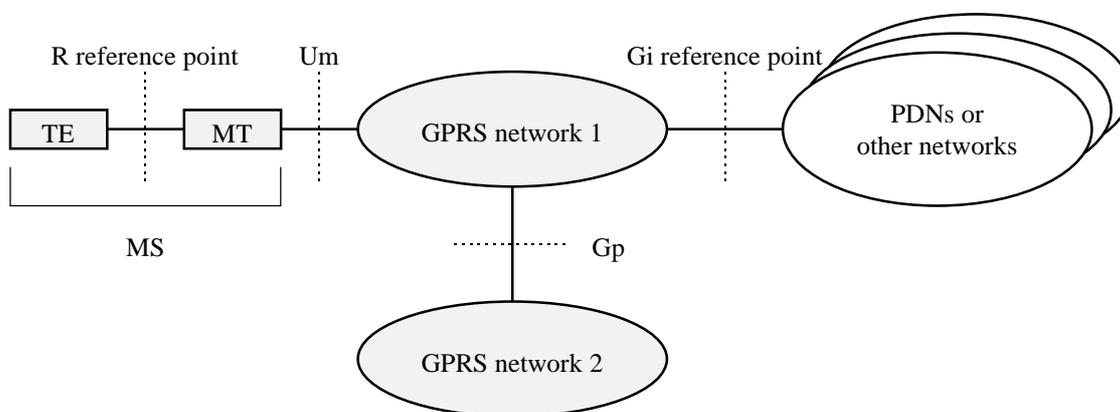
**Figure 1: GPRS Access Interfaces and Reference Points**
