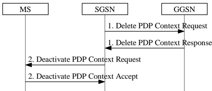
**Figure 42: PDP Context Deactivation Initiated by SGSN Procedure**
