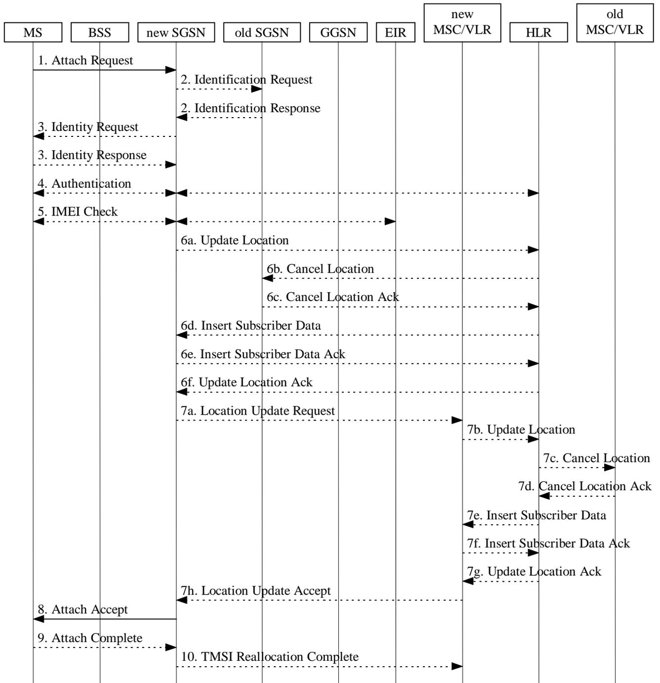
**Figure 1: Combined GPRS / IMSI Attach Procedure**
