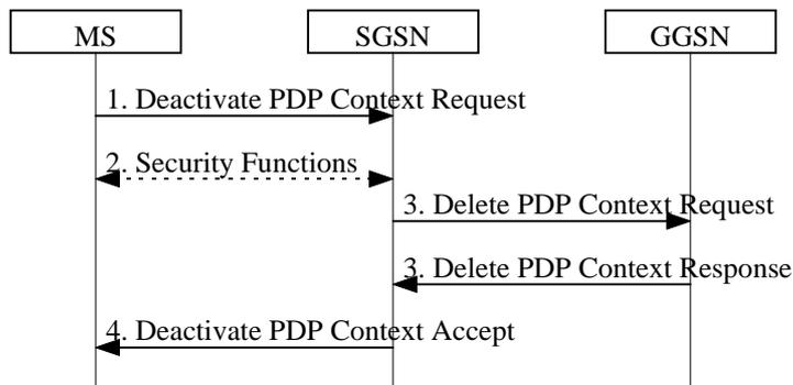
**Figure 40: PDP Context Deactivation Initiated by MS Procedure**
