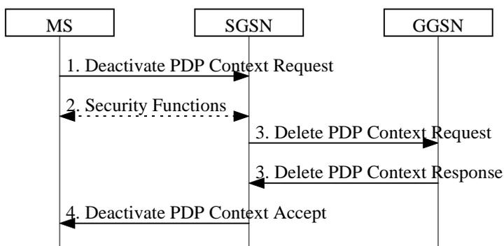
**Figure 41: PDP Context Deactivation Initiated by MS Procedure**
