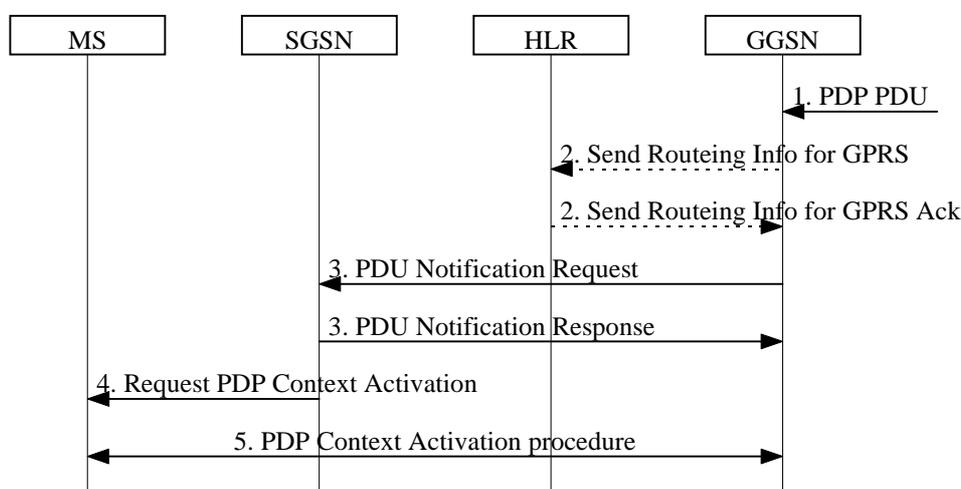
**Figure 35: Successful Network-Requested PDP Context Activation Procedure**
