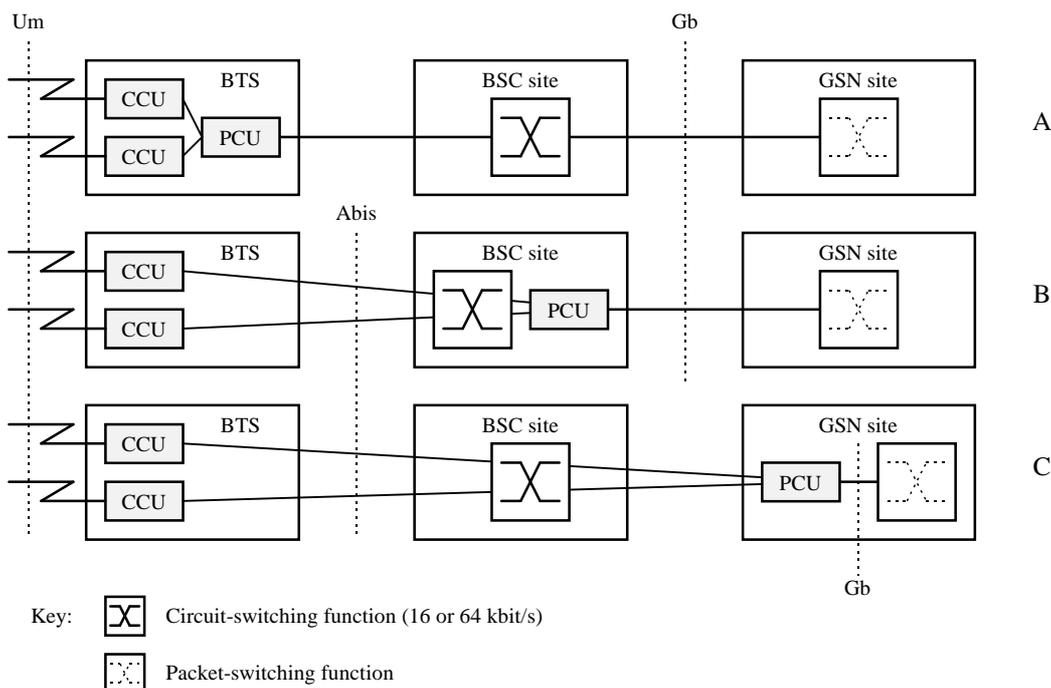
**Figure 48: Remote Packet Control Unit (PCU) Positions**
