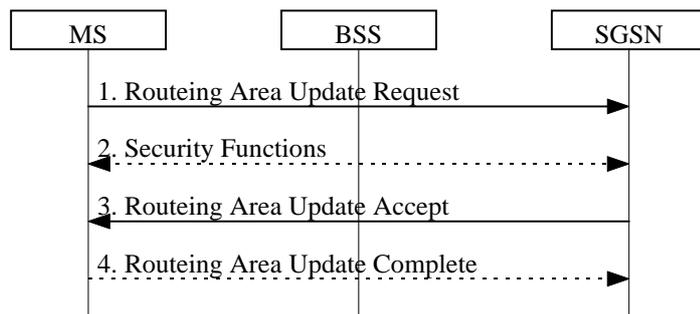
**Figure 27: Intra SGSN Routeing Area Update Procedure**
