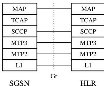
Figure 6: Signalling Plane SGSN - HLR
