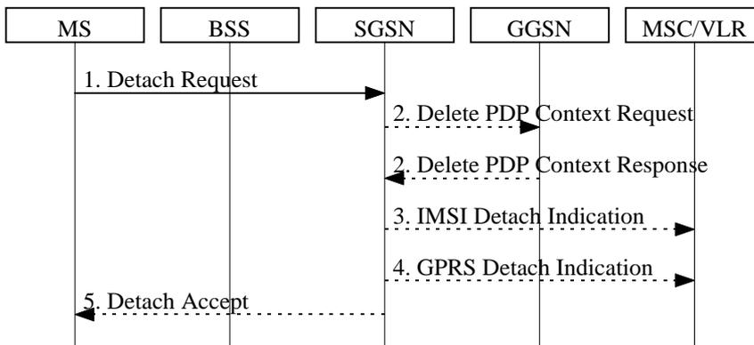
**Figure 19: MS-Initiated Combined GPRS / IMSI Detach Procedure**
