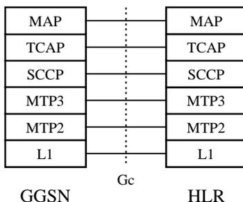
Figure 10: Signalling Plane GGSN - HLR Using MAP
