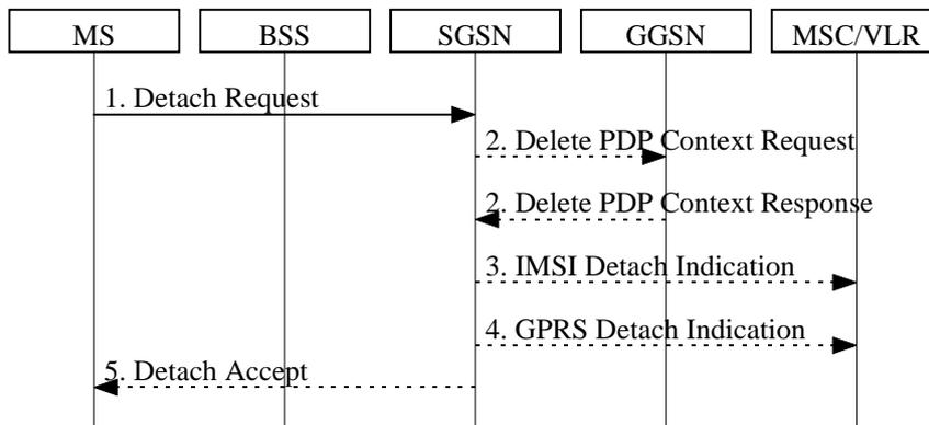
**Figure 18: MS-Initiated Combined GPRS / IMSI Detach Procedure**
