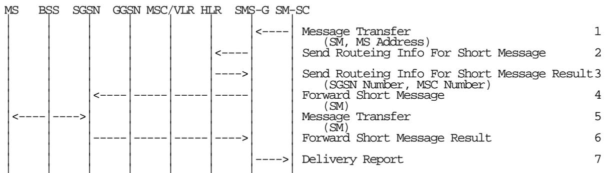
Figure 55: MT SMS Transfer, Successful
