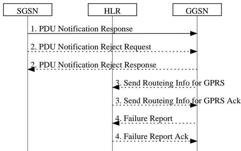
**Figure 37: Protection Procedure**
