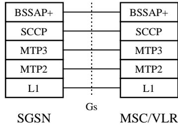
Figure 7: Signalling Plane SGSN - MSC/VLR
