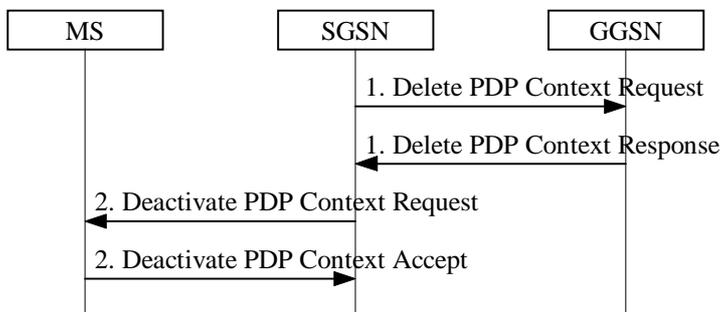
**Figure 41: PDP Context Deactivation Initiated by SGSN Procedure**
