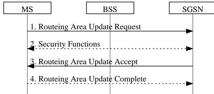
**Figure 2: Intra SGSN Routing Area Update Procedure**
