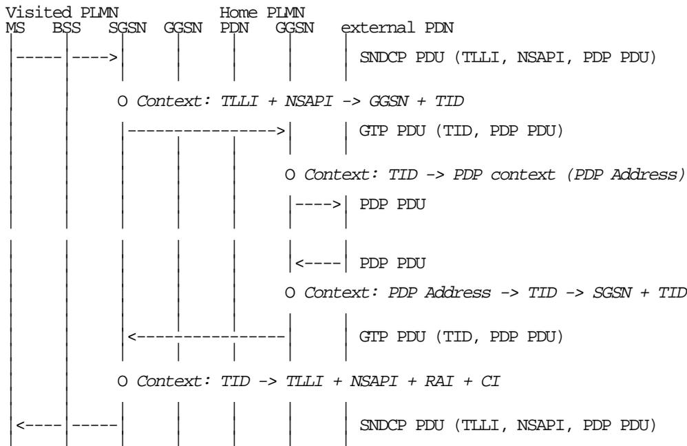
Figure C.2: Data Routeing for a Roaming MS to and from an External PDN
