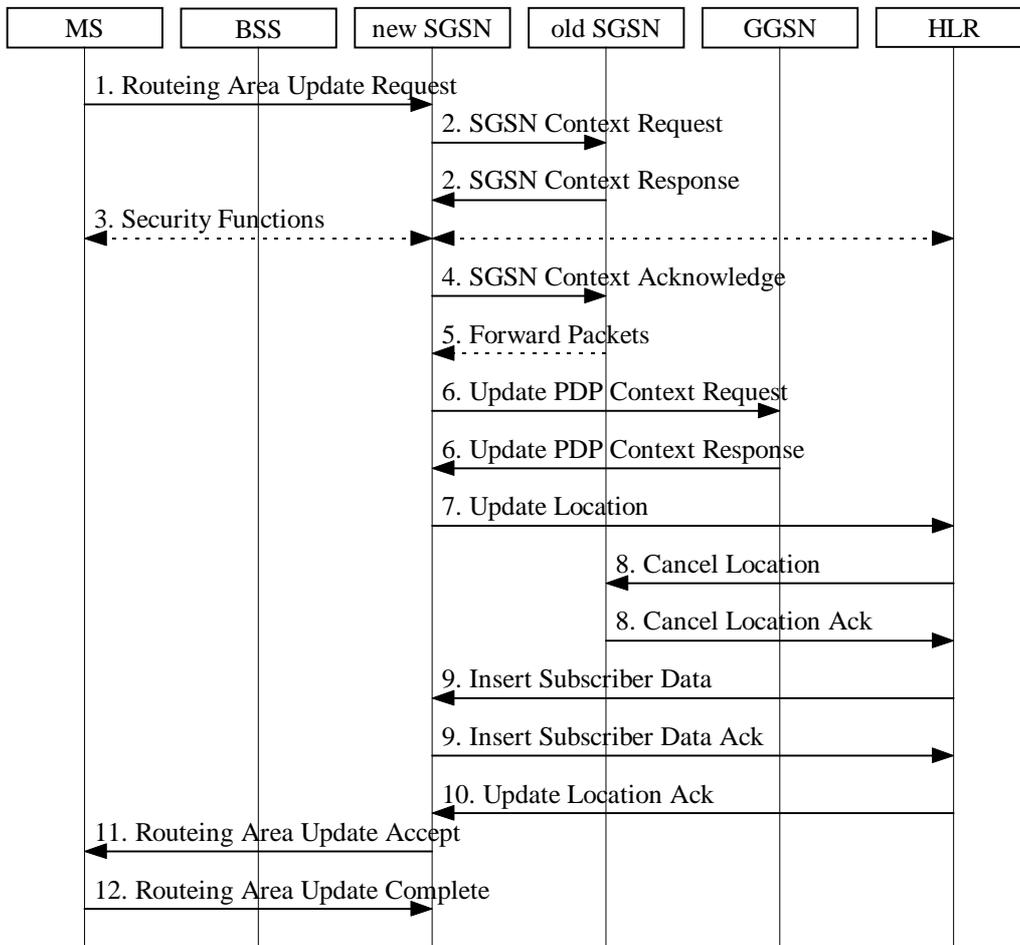
**Figure 27: Inter SGSN Routing Area Update Procedure**
