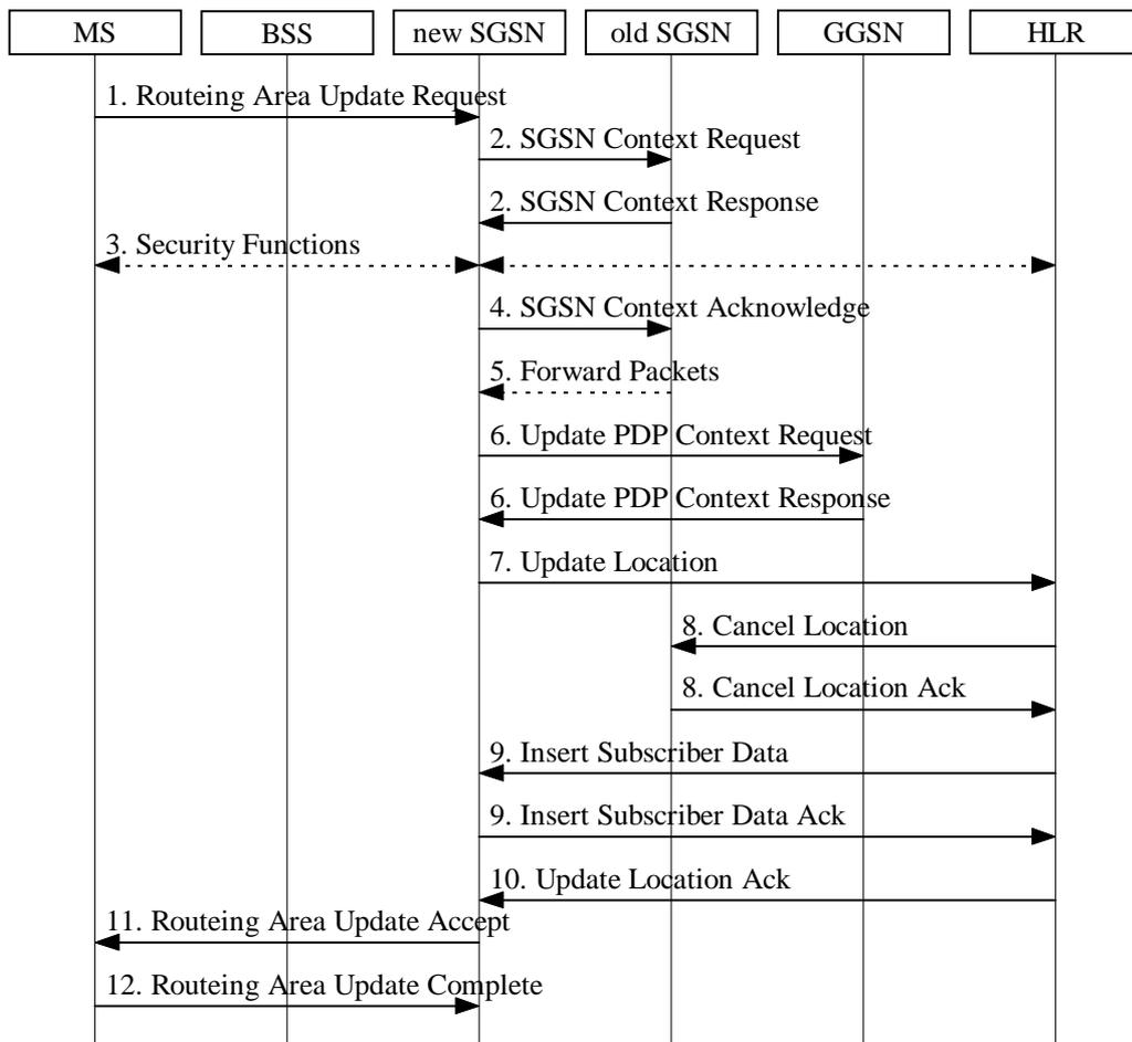
**Figure 3: Inter SGSN Routeing Area Update Procedure**
