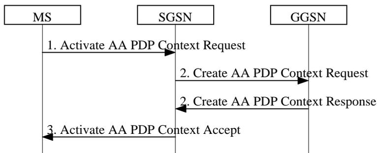
**Figure 39: Anonymous Access PDP Context Activation Procedure**
