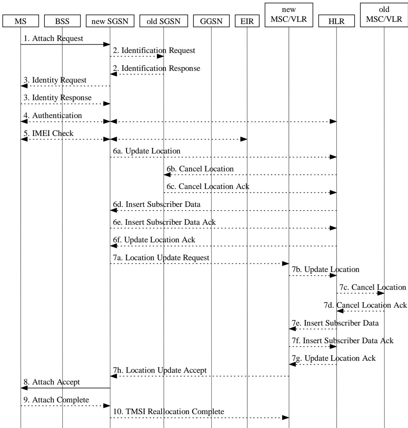
**Figure 18: Combined GPRS / IMSI Attach Procedure**
