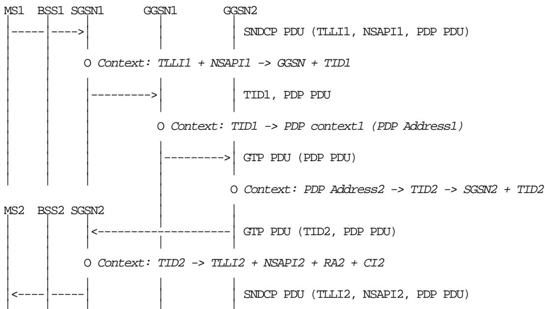
Figure C.4: MS-to-MS Data Routing via Different GGSNs
