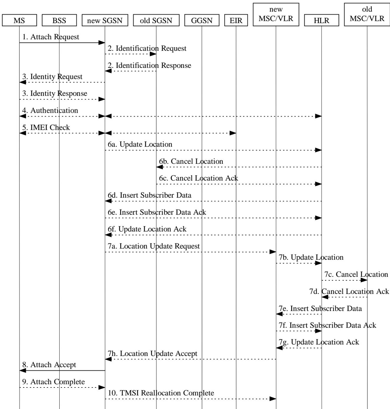
**Figure 17: Combined GPRS / IMSI Attach Procedure**
