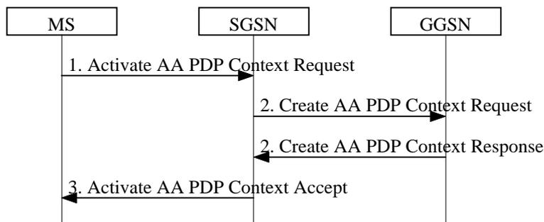
**Figure 2: Anonymous Access PDP Context Activation Procedure**
