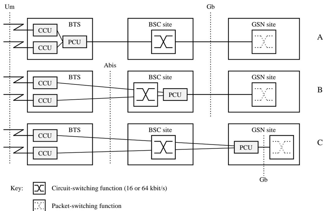
**Figure 51: Remote Packet Control Unit (PCU) Positions**
