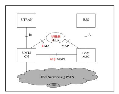
Figure xx. Inter-Operability between GSM and UMTS
