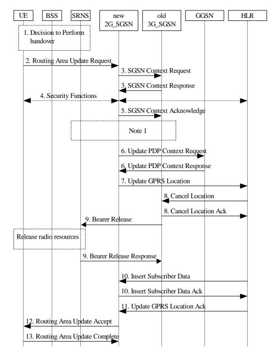
Figure 23: UMTS to GSM GPRS, Inter SGSN Routing Area Update Procedure
