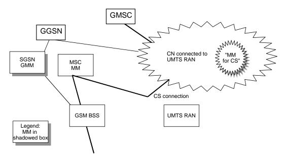
Figure 11 After HO from UMTS to GSM.
