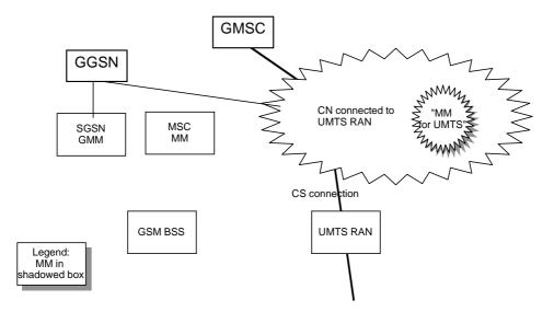
Figure 10 Before HO from UMTS to GSM.
