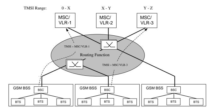
Figure 17: Example of GSM Turbo-Charger Network Architecture
