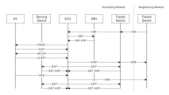
Figure 16. Signalling Flow for MT Call.
