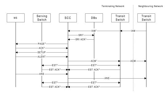
Figure 16. Signalling Flow for MT Call.
