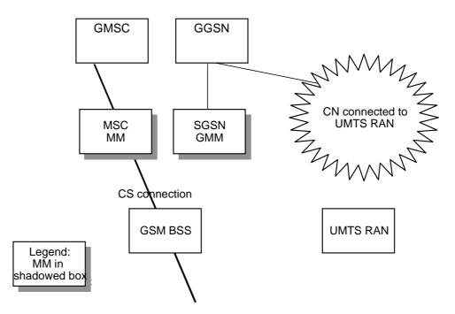
Figure 8. Before HO to UMTS from GSM. The PS services are provided from SGSN in GSM.
