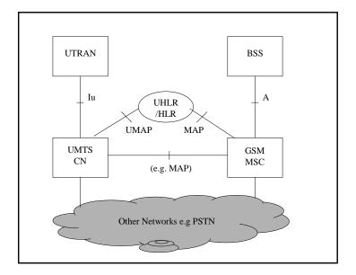
Figure xx. Inter-Operability between GSM and UMTS
