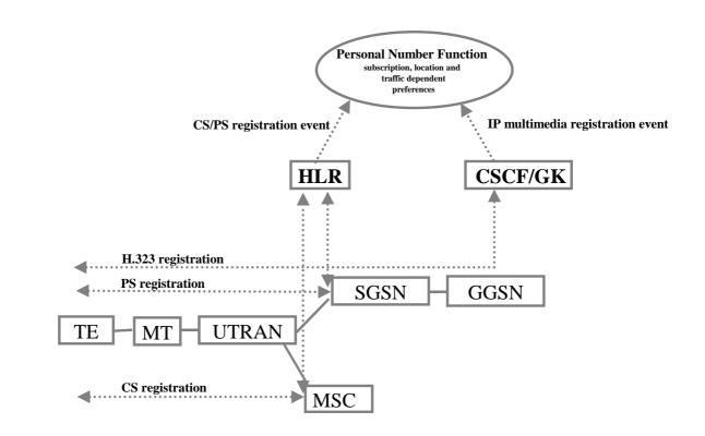
Above is shown how a CS/PS mobile terminal e.g. at power on makes three types of registrations. One is a circuit registration, one is a GPRS registration, and one is an IP multimedia e.g. H.323 registration. The latter is done within the GPRS user plane. The HLR indicates to the Personal Number Function that the user is available for CS speech calls. The CSCF indicates to the Personal Number Function that the user is available for IP multimedia voice calls.
