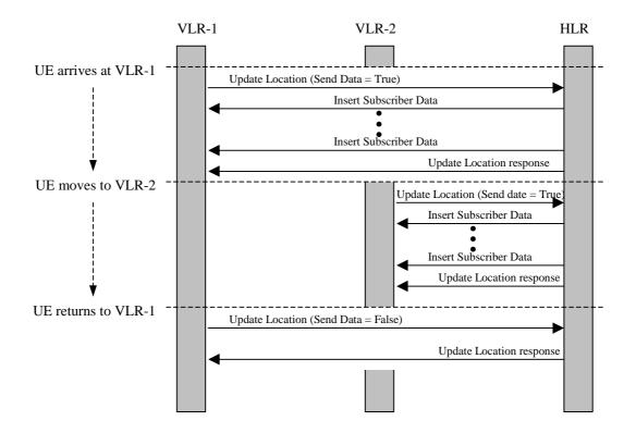
Figure 2: Example message flow in a Super-Charged network.
