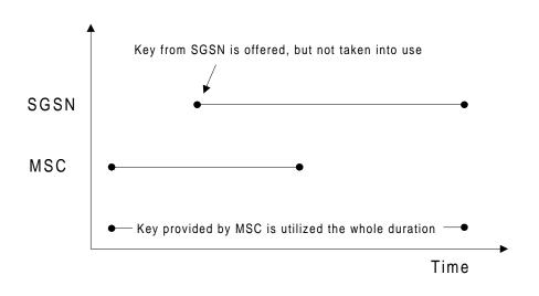
Figure 3. One ciphering key use in the UTRAN
