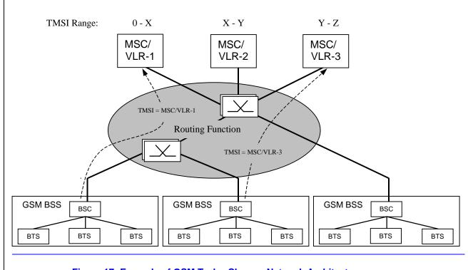
Figure 17: Example of GSM Turbo-Charger Network Architecture
