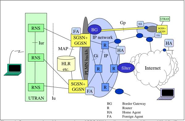
Figure 6. Core network architecture where GPRS MM handles active mobiles and Mobile IP streamlining at inter SGSN handover. The SGSN and GGSN are here co-located.
