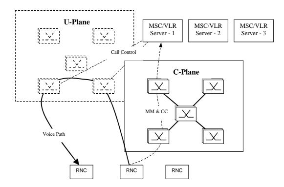
Figure 18: Example of UMTS Turbo-Charger Network Architecture
