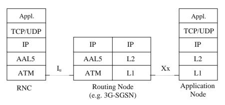
Figure XX: Protocol Stack of the Common Communication Channel
