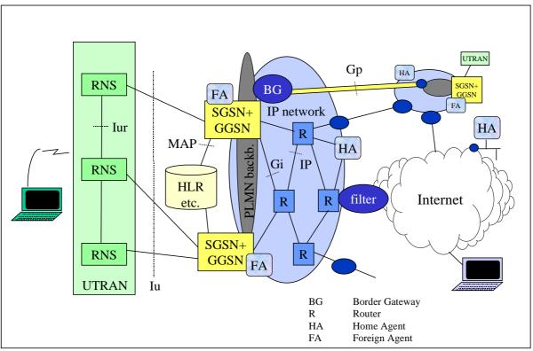
Figure 6. Core network architecture where GPRS MM handles active mobiles and Mobile IP streamlining at inter SGSN handover. The SGSN and GGSN are here co-located.
