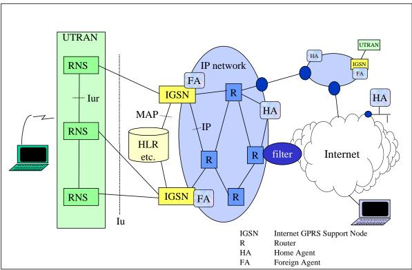
Figure 7. Core network architecture with Mobile IP MM within the CN and between different types of systems and between GPRS PLMN's.
