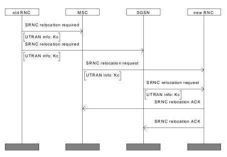
Figure 4. The ciphering key transfer in SRNC relocation procedure (one ciphering key)
