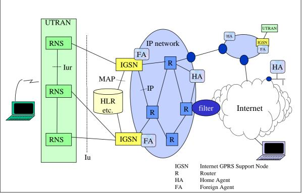
Figure 7. Core network architecture with Mobile IP MM within the CN and between different types of systems and between GPRS PLMN's.
