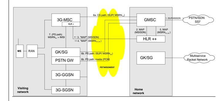
Step 7 could further be enhanced to provide subscriber information pertaining to supplementary services, hence allowing common services to be provided to the user, regardless of the path (CS or PS) used to route the call.
