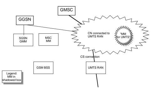
Figure 10 Before HO from UMTS to GSM.
