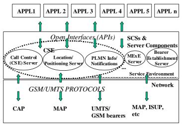
Fig. 3 UMTS standardised service capabilities
