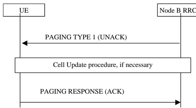
**Figure 222222) UTRAN originated paging procedure in connected mode**
