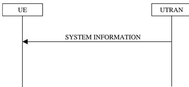
**Figure 333) Procedure for broadcast of system information**
