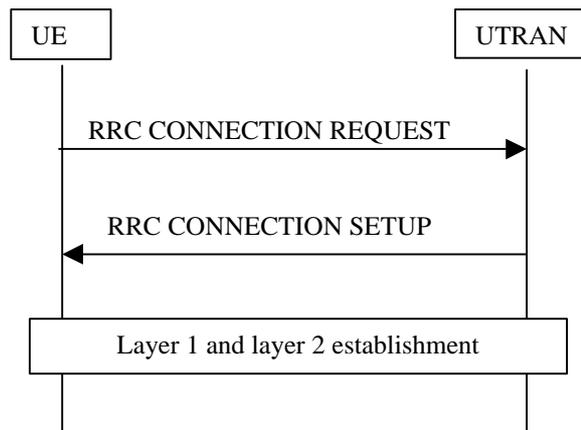
**Figure 666) Procedure for RRC connection establishment**
