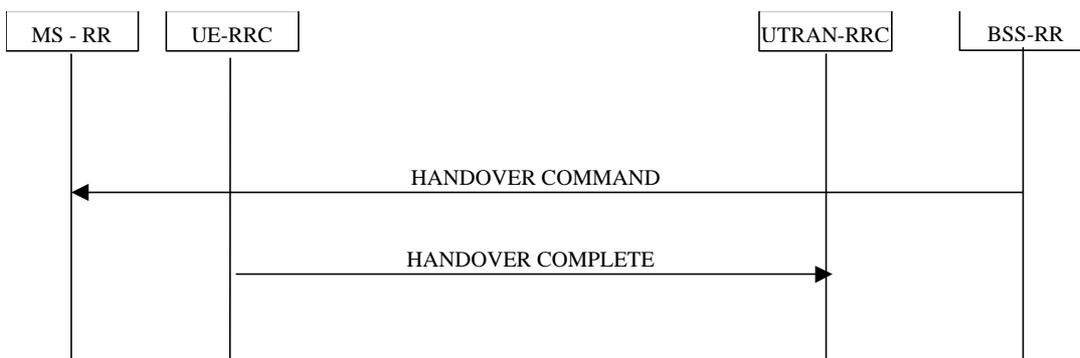
**Figure 1717** Procedure for Inter-system hard hand-over - GSM to UTRAN
