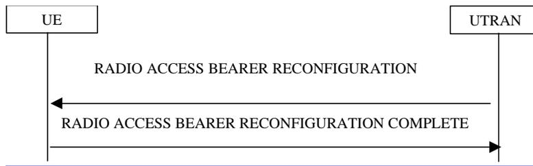
Figure 11.11) Radio Access Bearer and signalling link Reconfiguration Procedure
