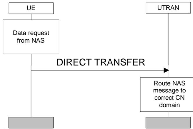
Figure 272727) Direct Transfer procedure in uplink
