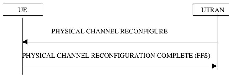
**Figure 1414** Physical Channel Reconfiguration procedure
