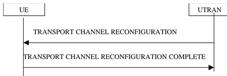
Figure 12.12) Procedure for transport channel reconfiguration
