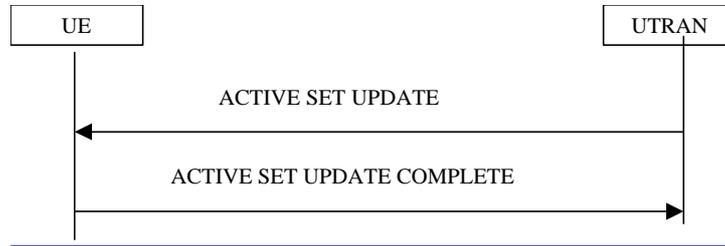
**Figure 15.15) Procedure for modifying the active set when in soft hand-over**
