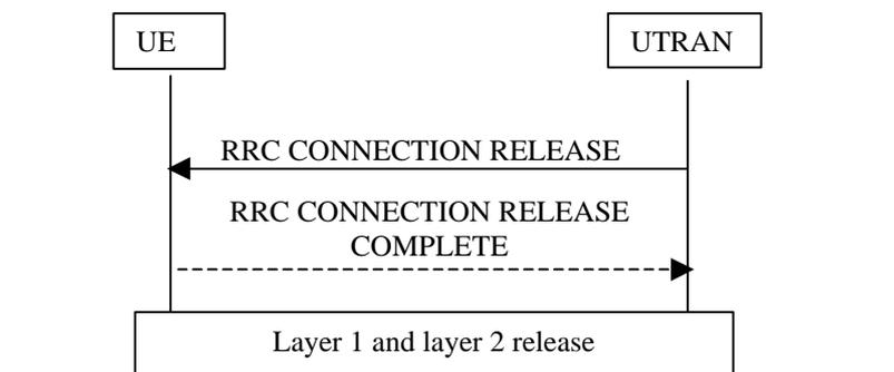
**Figure 777) RRC Connection release procedure**
