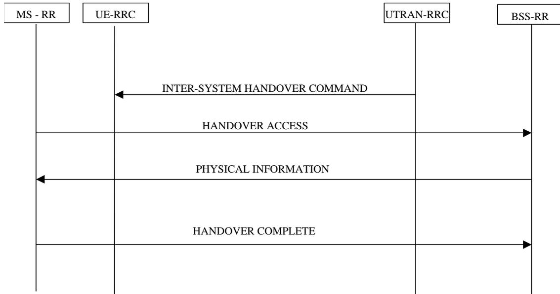
**Figure 181818) Inter system hard hand-off (UTRAN to GSM/BSS), PSTN/ISDN services**
