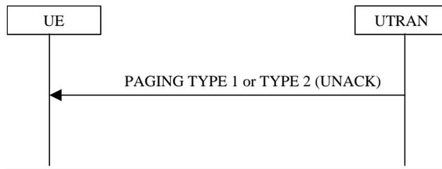
**Figure 212121) Core network originated paging procedure in connected mode**
