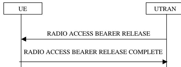
Figure ~~1010~~10) Radio Access Bearer Release Procedure
