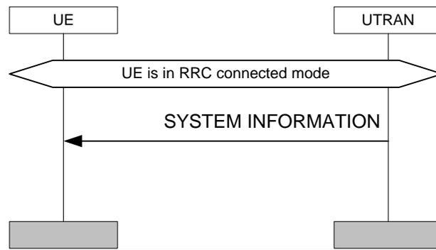
Figure 26.26) Sending of system information to UE in RRC connected mode
