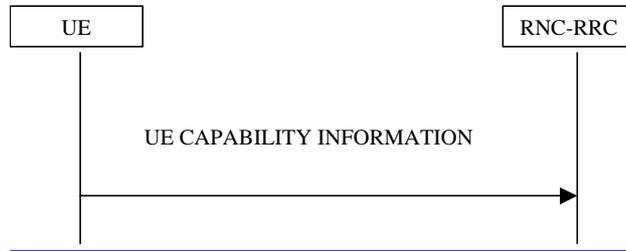
Figure 25.25) Procedure for transmission of UE capability information
