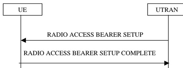
**Figure 999) Radio Access Bearer Establishment Procedure**
