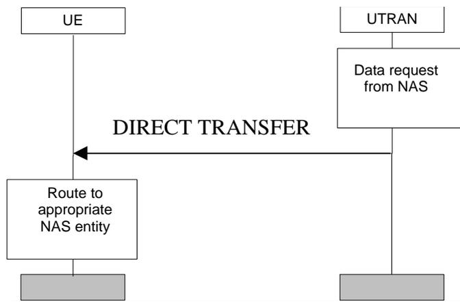
Figure 282828) Direct Transfer procedure in downlink
