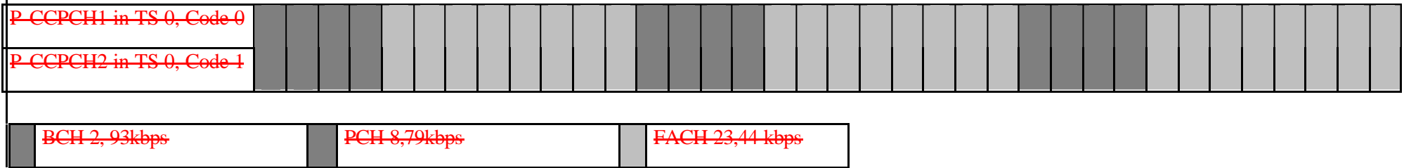
Figure B.1: Example for a multiframe structure for P-CCPCHs that is repeated every 72th frame (144 sub-frame)
