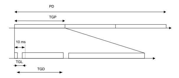
Figure 1: illustration of compressed mode pattern parameters
