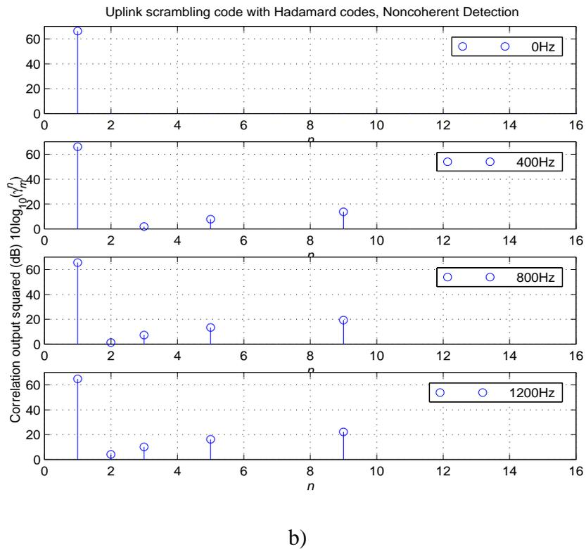
**Figure 4: Decision statistics for noncoherent detection with a) present non-differentially encoded preambles and b) proposed preambles.**
