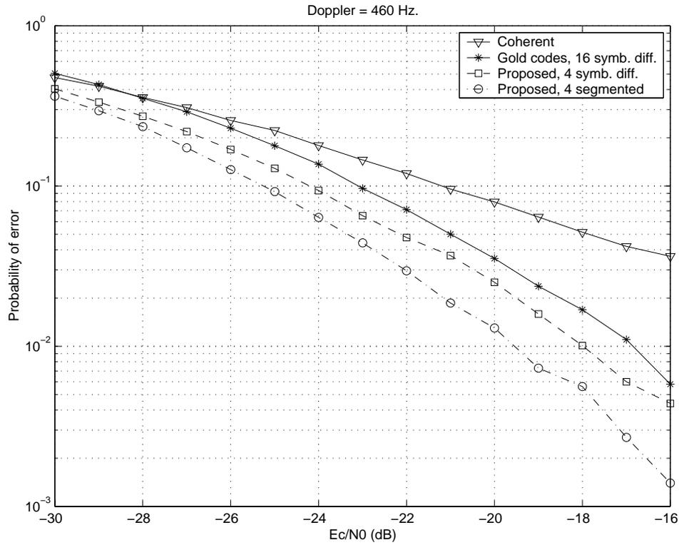
**Figure 25: Probability of maximum decision statistic not corresponding to transmitted preamble. Fading channel, 250 km/h with a 2 GHz carrier frequency.**
