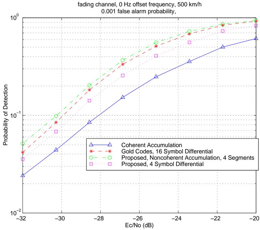
**Figure 19: Fading channel detection performance. 500 km/h**
