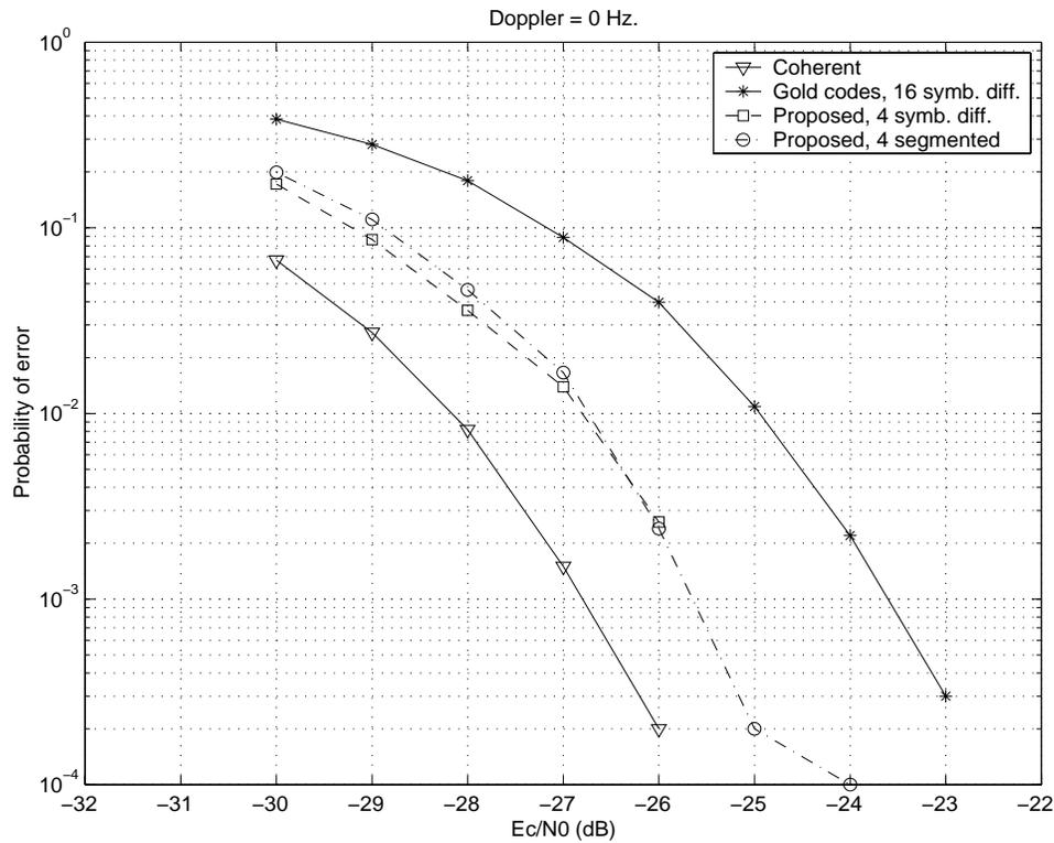
**Figure 24: Probability of maximum decision statistic not corresponding to transmitted preamble. Fading channel, fading constant across preamble.**
