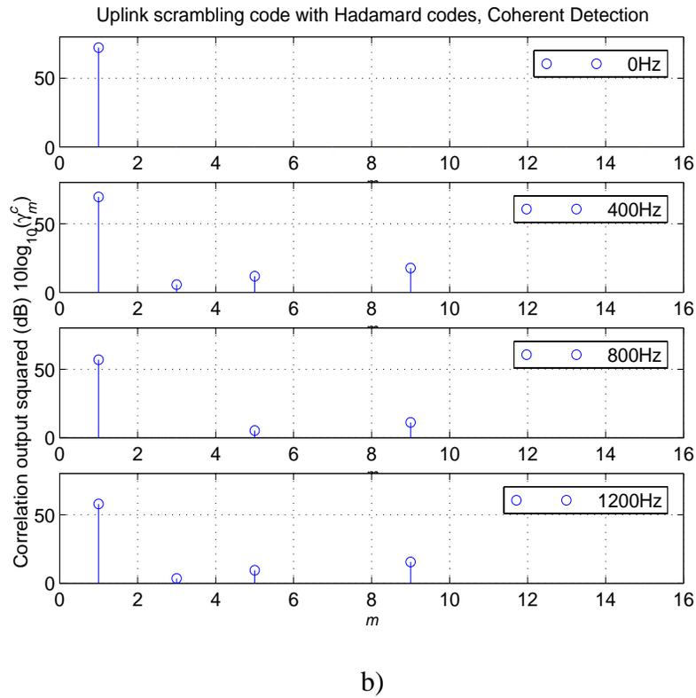
**Figure 3: Decision statistics for coherent detection with a) present preamble and b) proposed preambles.**
