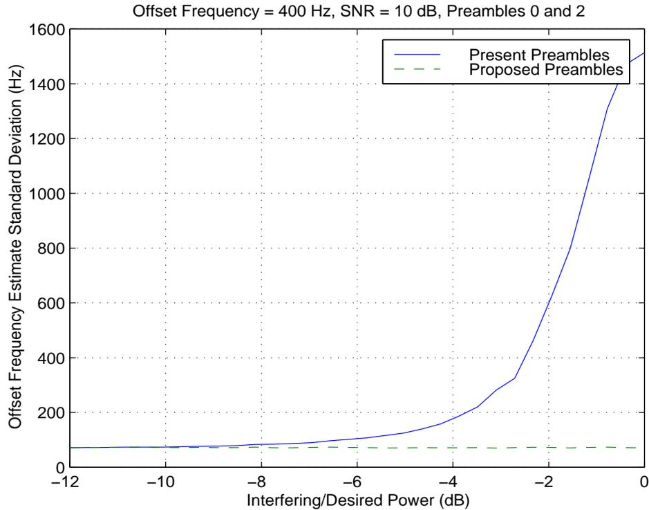
**Figure 7: Effect of interfering preamble on offset frequency estimation**
