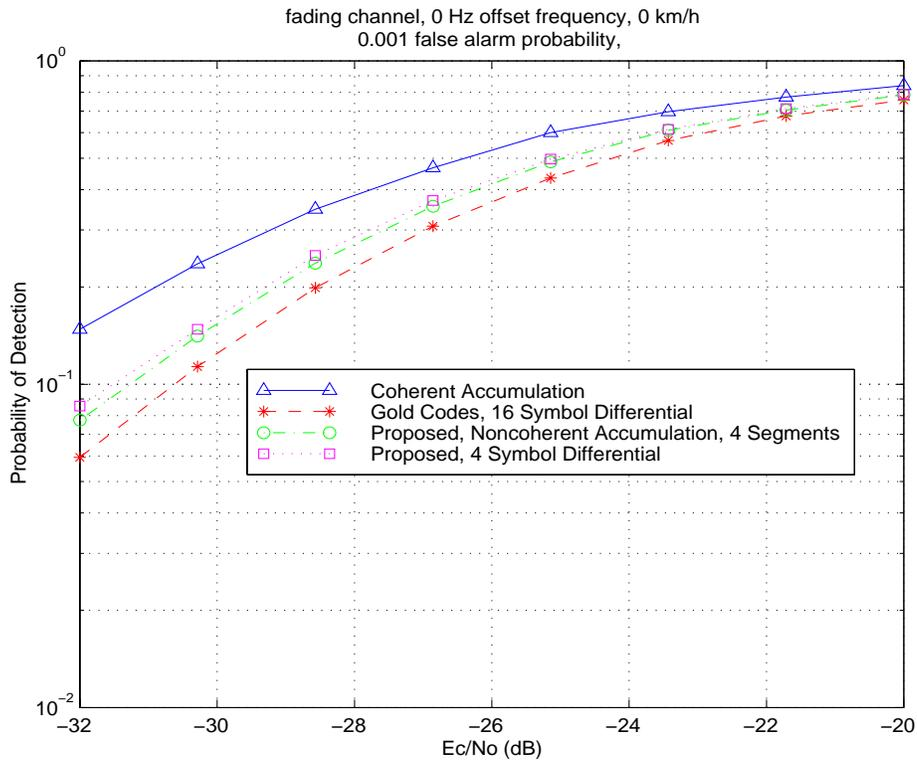
**Figure 15: Fading channel detection performance. Fading is constant across preamble.**
