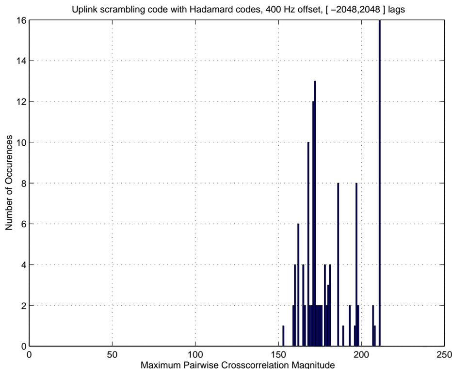
**Figure 6: Maximum absolute crosscorrelations for the proposed preambles when a channel phase rotation of 400 Hz is present.**
