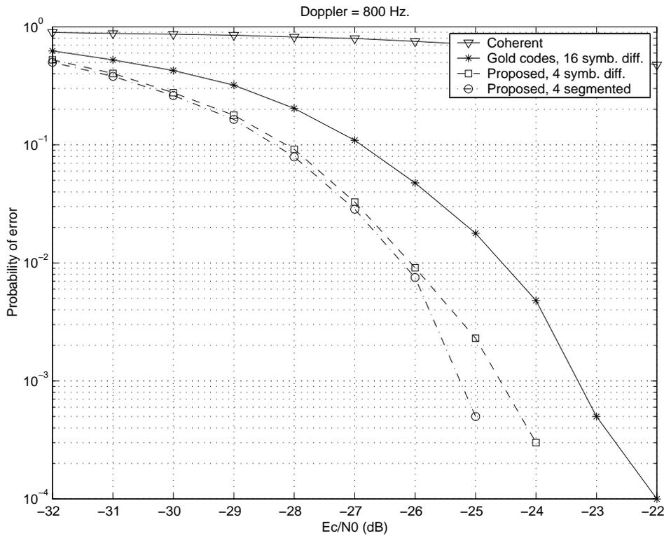
**Figure 22: Probability of maximum decision statistic not corresponding to transmitted preamble. Static channel, 800 Hz offset.**
