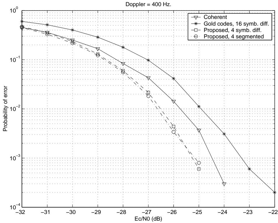
**Figure 21: Probability of maximum decision statistic not corresponding to transmitted preamble. Static channel, 400 Hz offset**
