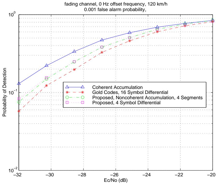
**Figure 17: Fading channel detection performance. 120 km/h**
