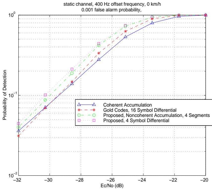
**Figure 12: Static channel detection performance. 400 Hz frequency offset.**
