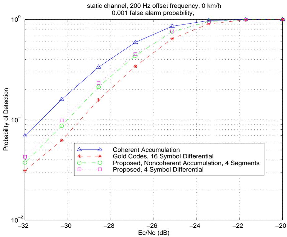
**Figure 11: Static channel detection performance. 200 Hz frequency offset.**
