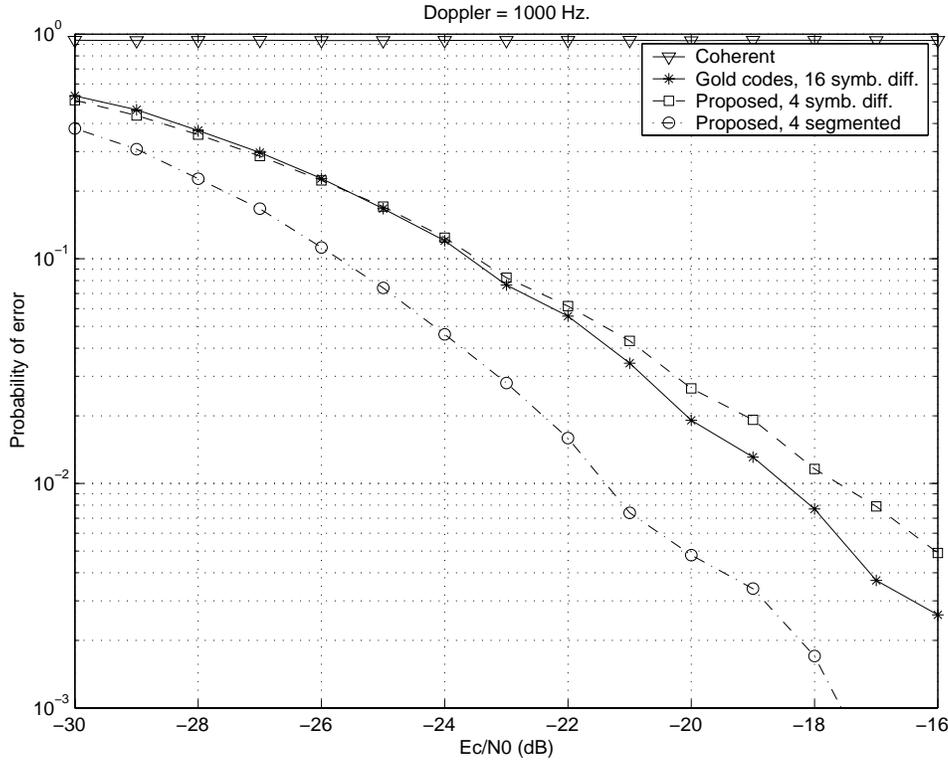
**Figure 27: Probability of maximum decision statistic not corresponding to transmitted preamble. Fading channel, 540 km/h with a 2 GHz carrier frequency**
