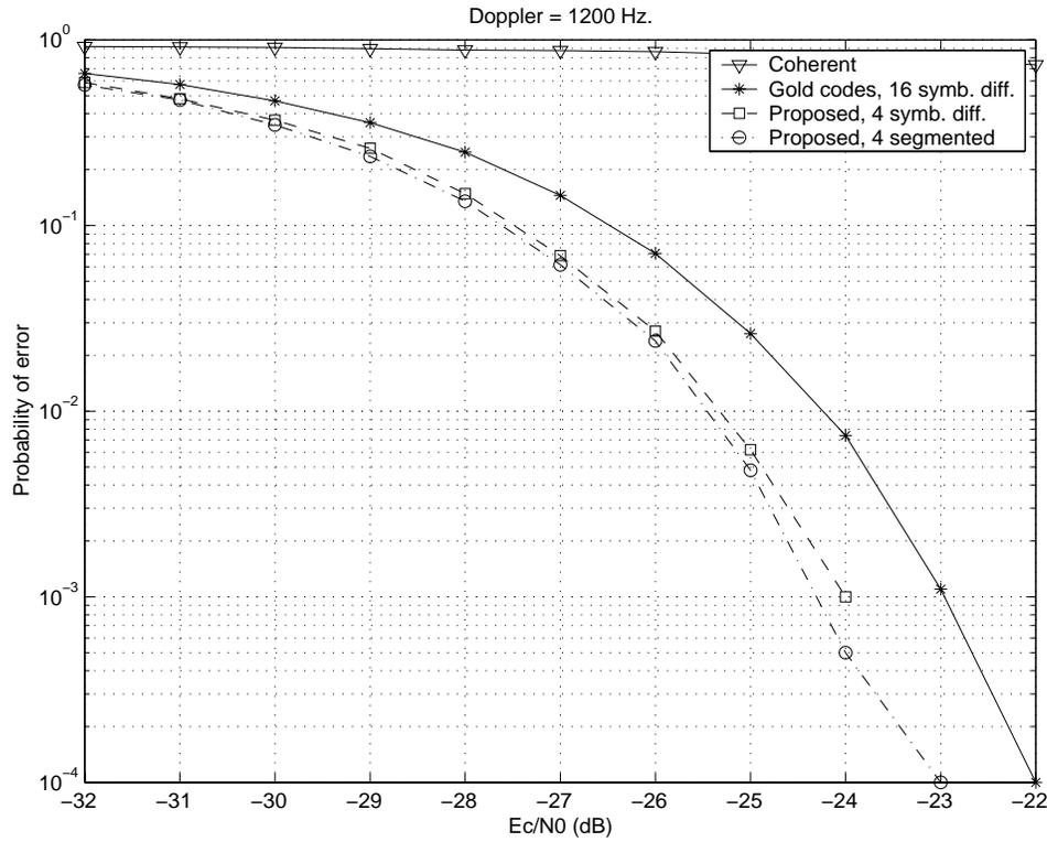
**Figure 23: Probability of maximum decision statistic not corresponding to transmitted preamble. Static channel, 1200 Hz offset.**
