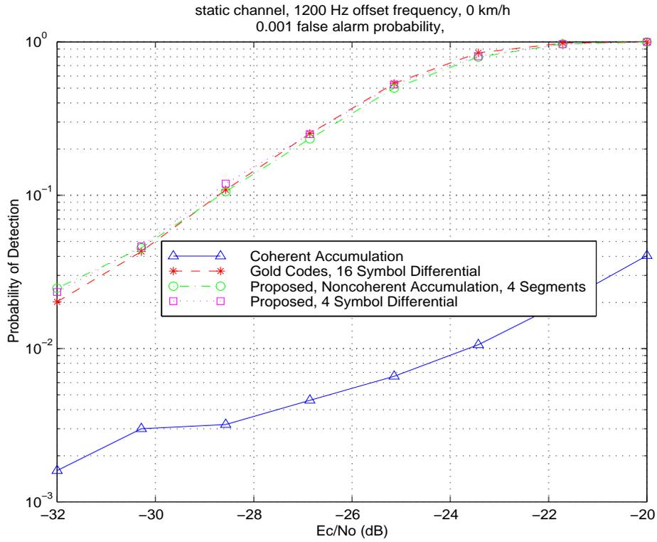
**Figure 14: Static channel detection performance. 1200 Hz frequency offset.**
