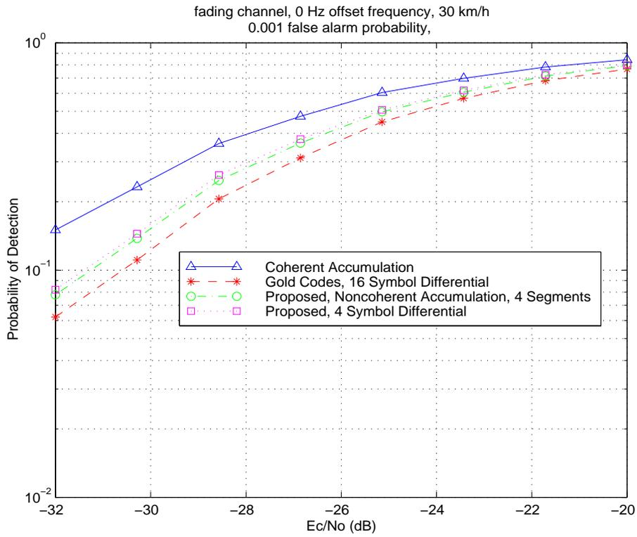
**Figure 16: Fading channel detection performance. 30 km/h**
