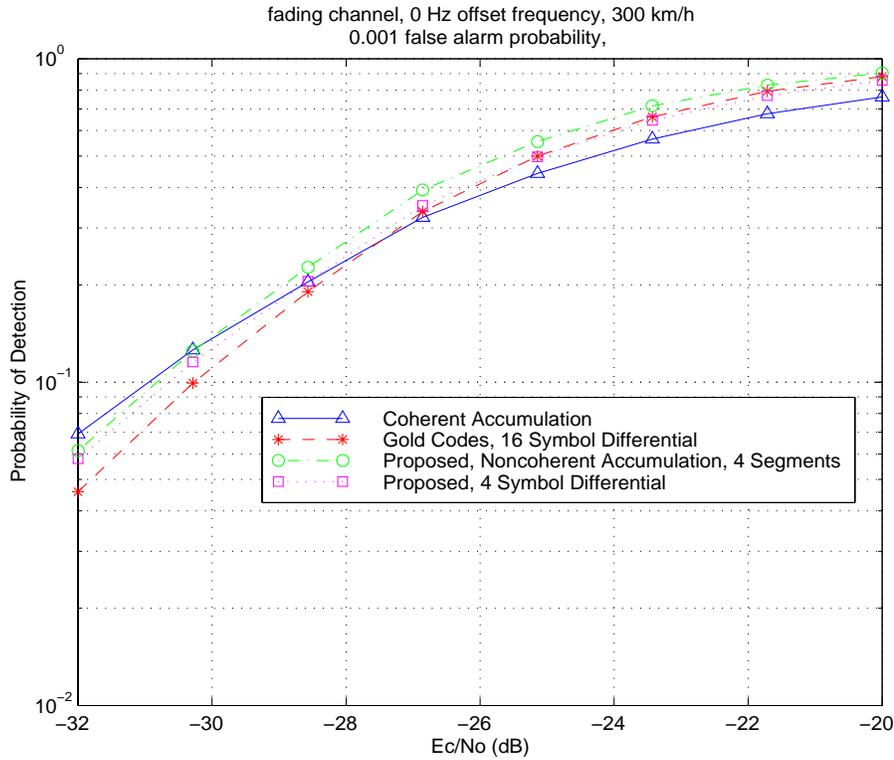
**Figure 18: Fading channel detection performance. 300 km/h**
