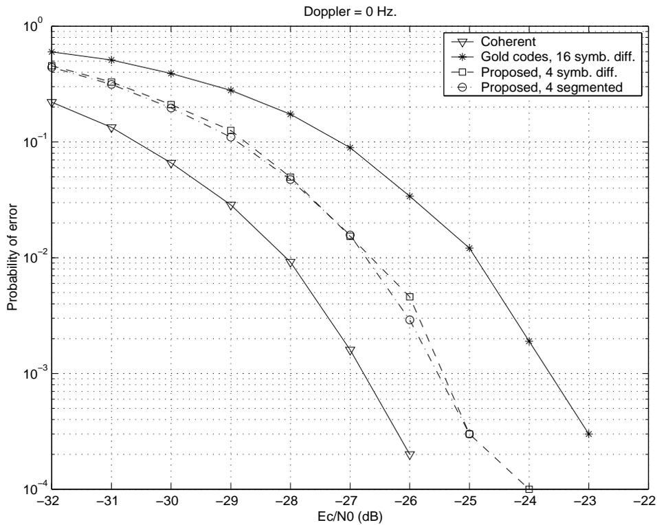
**Figure 20: Probability of maximum decision statistic not corresponding to transmitted preamble. Static channel, no frequency offset.**
