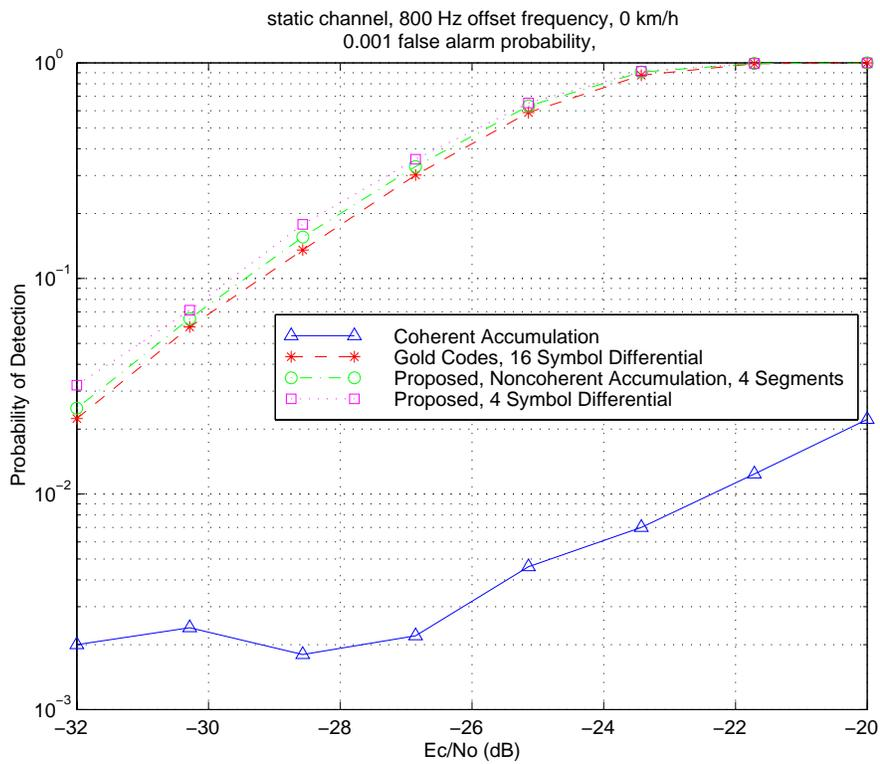
**Figure 13: Static channel detection performance. 800 Hz frequency offset.**
