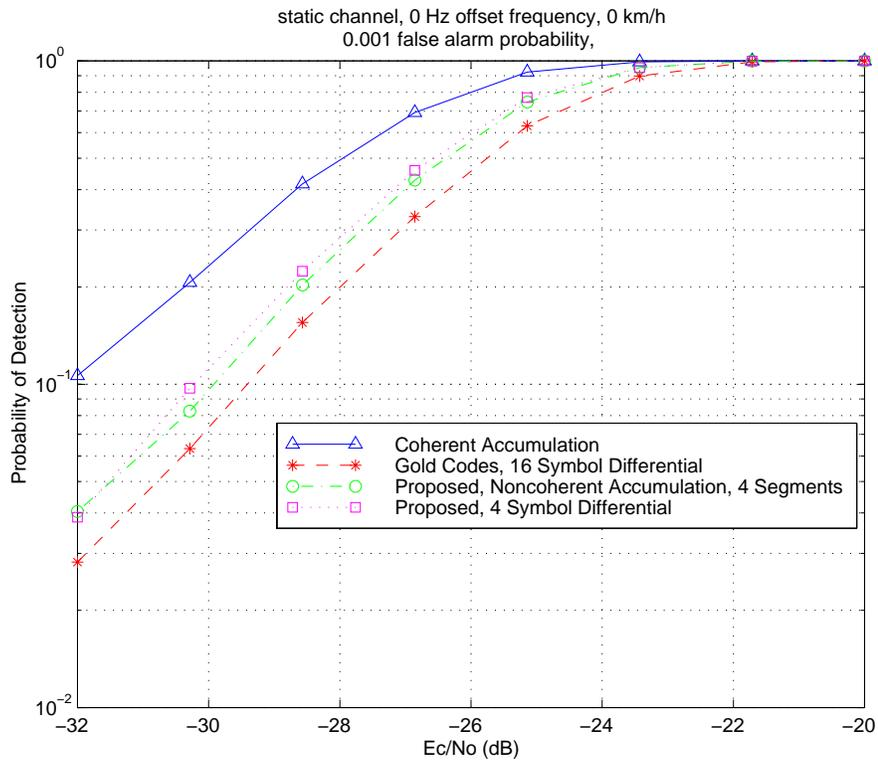
**Figure 10: Static channel detection performance. No frequency offset.**
