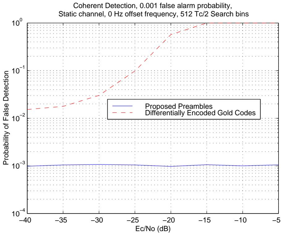
**Figure 29: Probability of false detection when coherent detection is performed on present differentially encoded preambles.**
