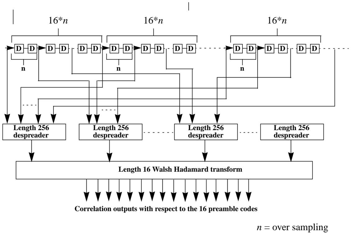
**Figure 9:** Figure 2: Block diagram of the preamble coherent receiver for the proposed Walsh Hadamard code based preamble. Due to the presence of a length 4096 long code on the top, a length  $4096*n$  matched filter is required,  $n$  being the amount of over sampling and is assumed to be 2 in the complexity calculations for this report.
