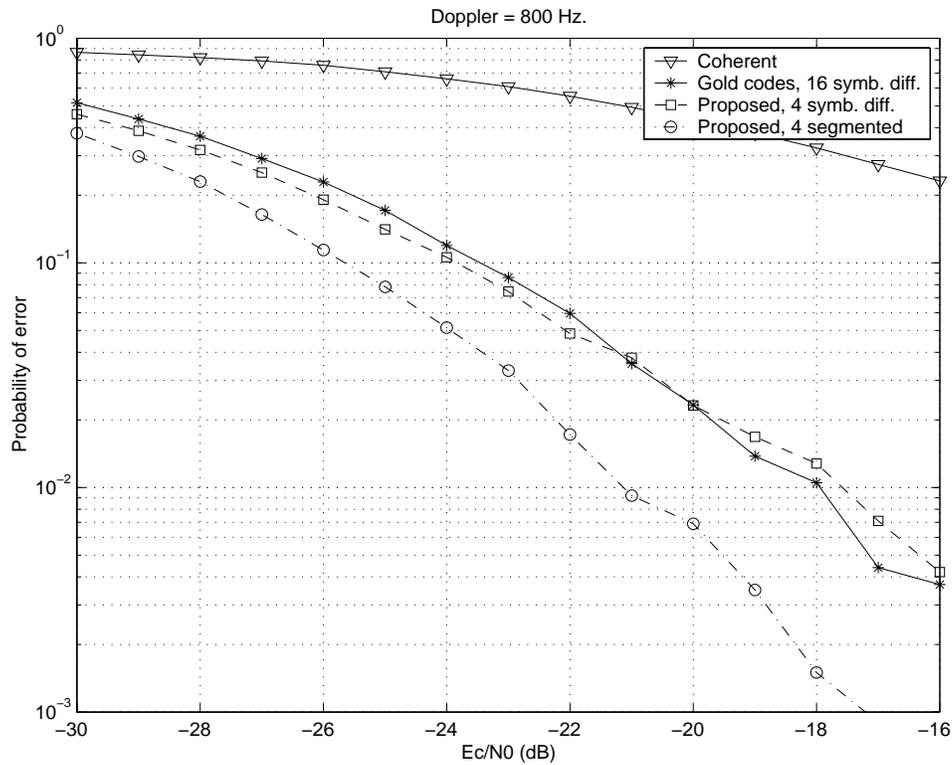
**Figure 26: Probability of maximum decision statistic not corresponding to transmitted preamble. Fading channel, 430 km/h with a 2 GHz carrier frequency**
