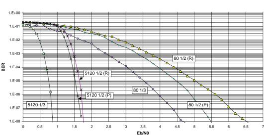
Simulation results - 4 SCCC -AWGN Channel
