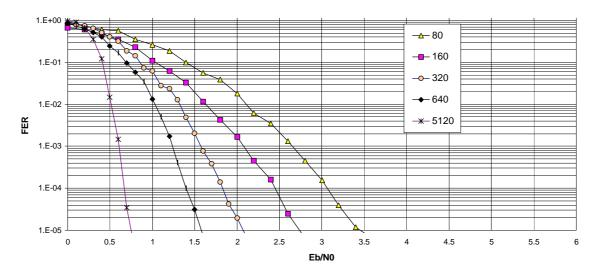
Figure 5: Frame error probability of the 4-state SCCC over the AWGN channel with a maximum of 100 iterations. Information block sizes: 40, 80, 160, 320, 640, and 5120.
