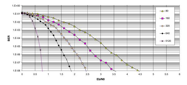
Figure 7: Bit error probability of the 4-state SCCC over the AWGN channel with a maximum of 100 iterations. Information block sizes: 80, 160, 320, 640, and 5120.
