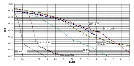
Figure 14: Bit error probability of the 8-state PCCC for block sizes of 80 and 5120 in the presence of random and periodic puncturing leading to a rate ½ code. The curves for rate 1/3 (unpunctured) is also reported.
