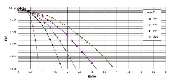
Simulation results - 4 SCCC - AWGN Channel
