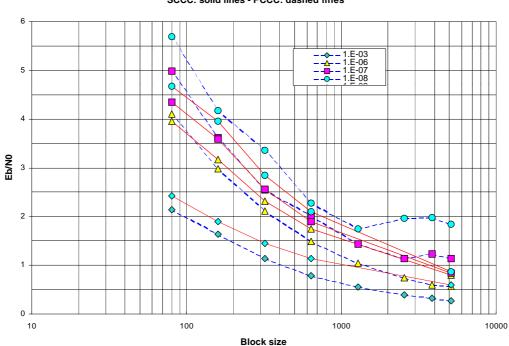
Eb/N0 for different QoS (BER) and different Block sizes SCCC: solid lines - PCCC: dashed lines
