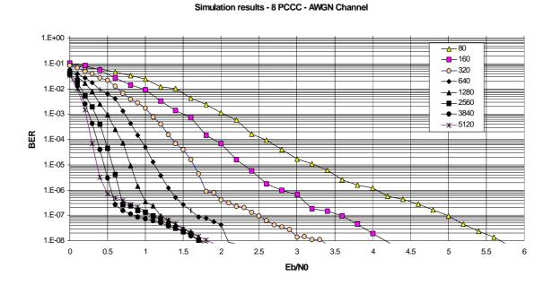
Figure 8: Bit error probability of the 8-state PCCC over the AWGN channel with a maximum of 100 iterations. Information block sizes: 80, 160, 320, 640, 1280, 2560, 3840, and 5120.
