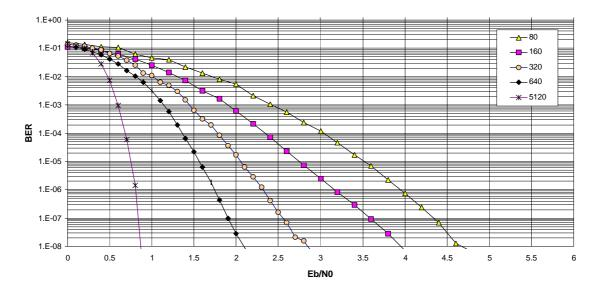
Figure 3: Bit error probability of the 4-state SCCC over the AWGN channel with a maximum of 10 iterations. Information block sizes: 80, 160, 320, 640, and 5120.
