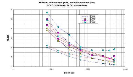
*Figure 12: Eb/N0 for different QoS (BER) and different Block sizes with a maximum of 100 iterations.*
