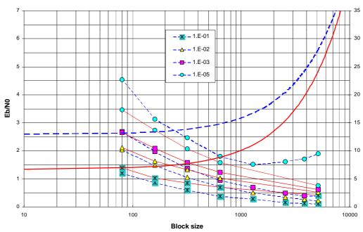
Eb/N0 for different QoS (FER) and different Block sizes SCCC: solid lines - PCCC: dashed lines
