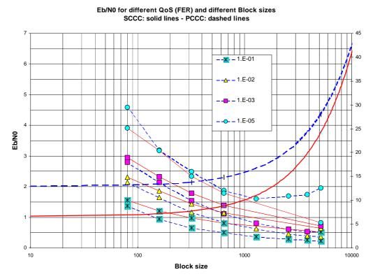
Figure 9: *Eb/N0* for different *QoS* (FER) and different Block sizes with a maximum of 10 iterations. The RHS ordinate reports the ASIC implementation complexity in square millimetres.
