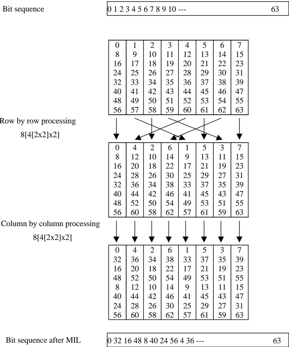
Fig. 1 An example of FS-MIL processing for 64 bits sequence.
