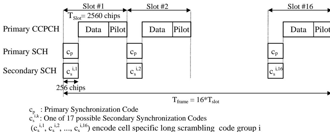
**Figure 3: Structure of Synchronisation Channel (SCH).**
