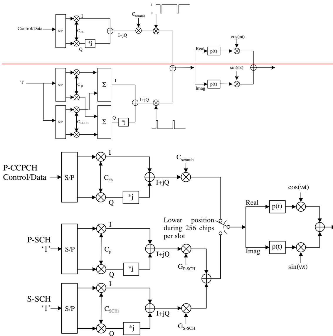
Figure 5. [Multiplexing of SCH]{Transmission of Perch Channel}
