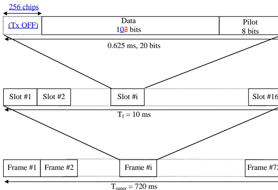
Figure 1: Frame structure for Primary Common Control Physical Channel.
