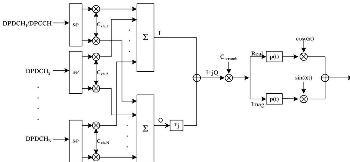
Figure 4. Spreading/modulation for downlink DPCH and CCPCHs.
