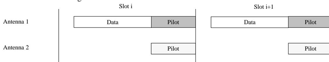
Figure 2: Slot structure of Primary CCPCH when diversity transmission is applied on dedicated channels.
