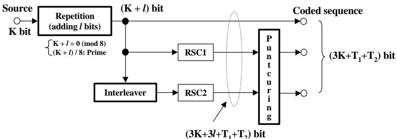
**Fig. 2** Block diagram of turbo encoder.
