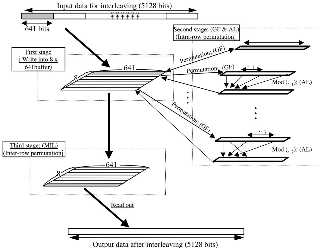
**Fig. 1** Block diagram of the merger interleaver.
