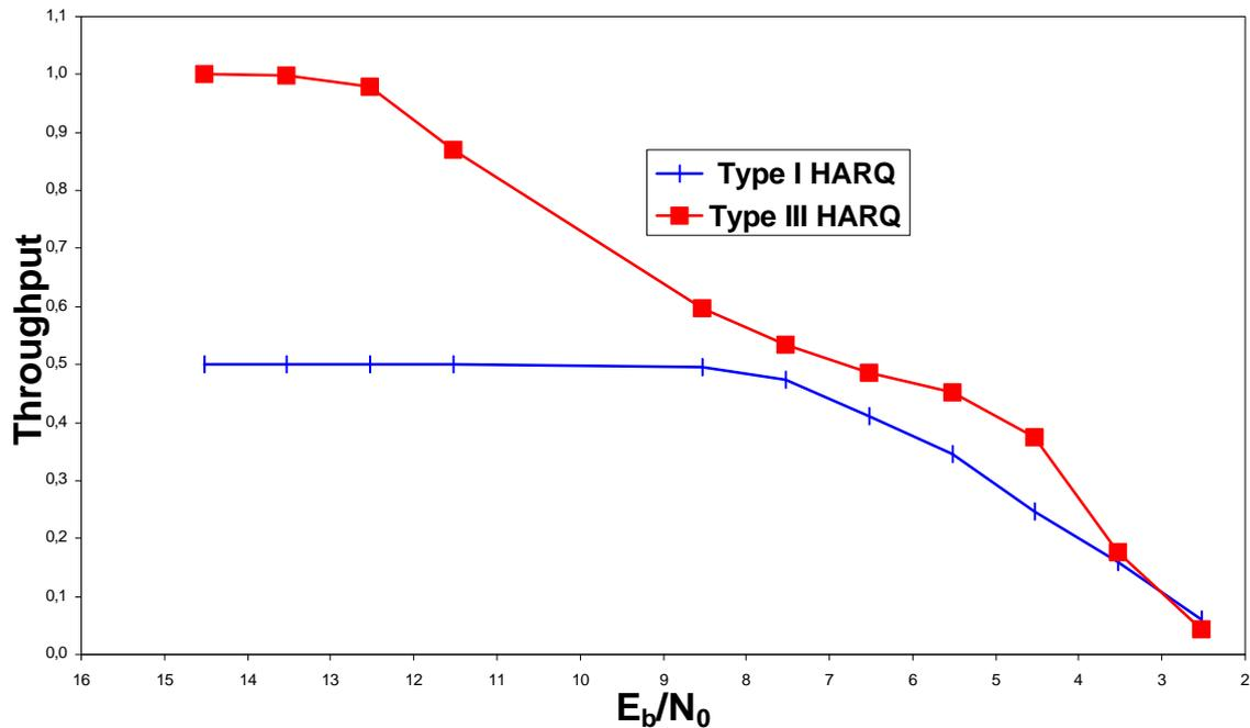
**Figure 2: Throughput of hybrid ARQ Type I and III**
