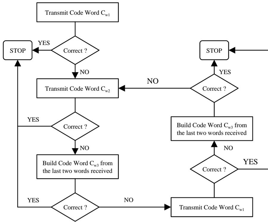
**Figure 1: Type III Hybrid ARQ transmission flow**
