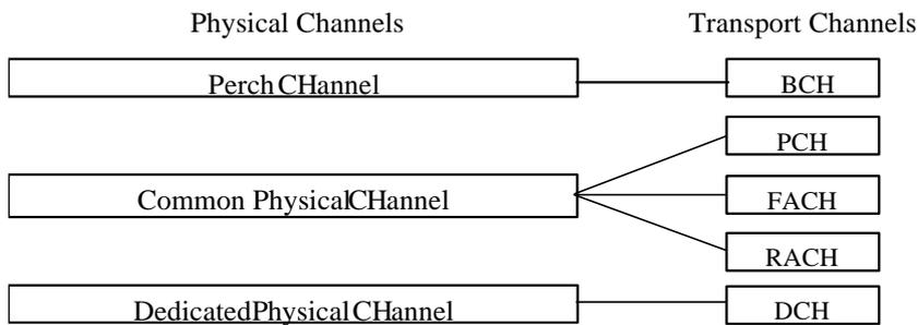
Fig. 3.2.1-5 Correspondence between Physical Channels and Transport Channels
