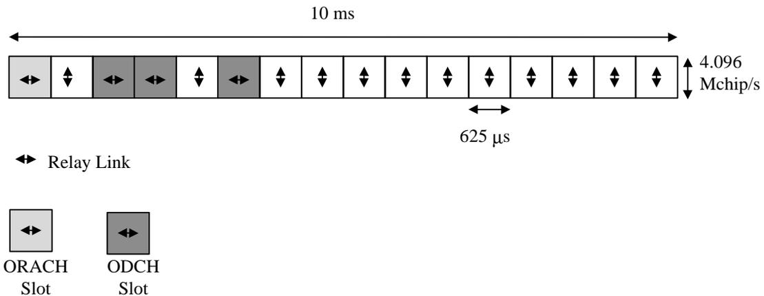
**Figure 4 TDD frame structure example for ODMA operation.**
