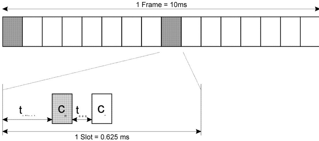
**Figure 9 Scheme for Synchronisation channel SCH consisting of one primary sequence  $C_p$  and one secondary sequence  $C_s$  per used slot**
