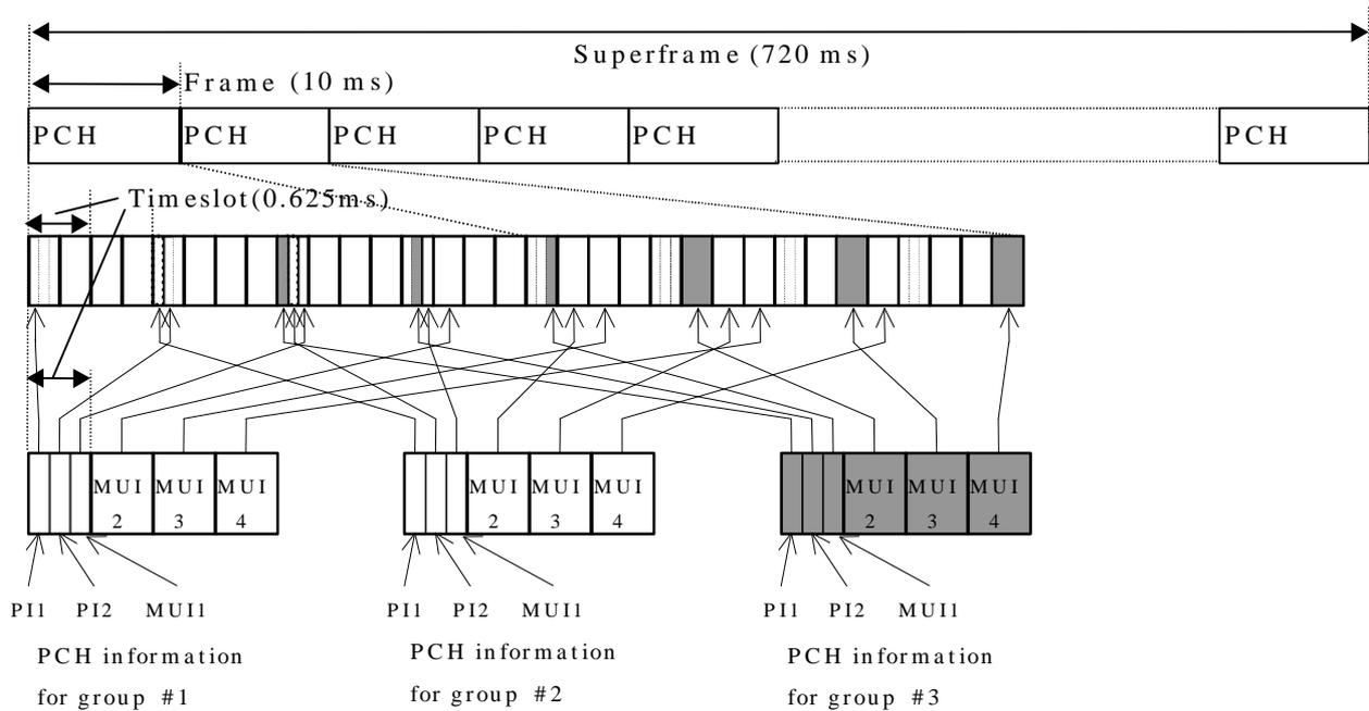
Fig. 3.3.1-1 PCH Mapping Method (example)
