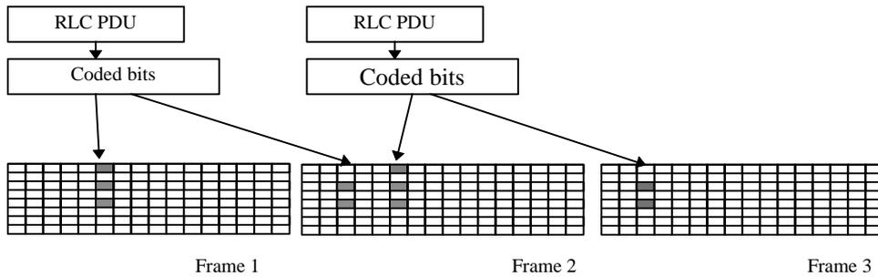
**Figure 12 Mapping of PDU onto the physical bearer**
