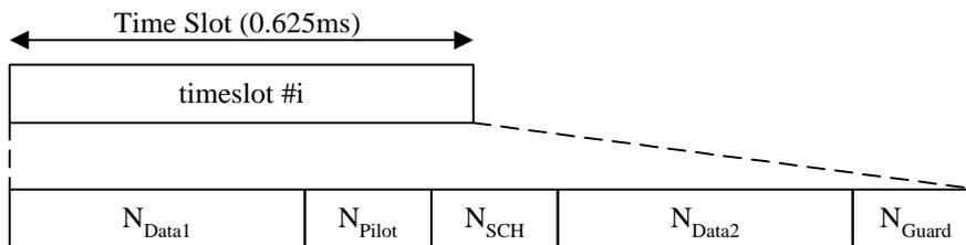
Fig.3.3.2-2 Perch Channel Signal Format
