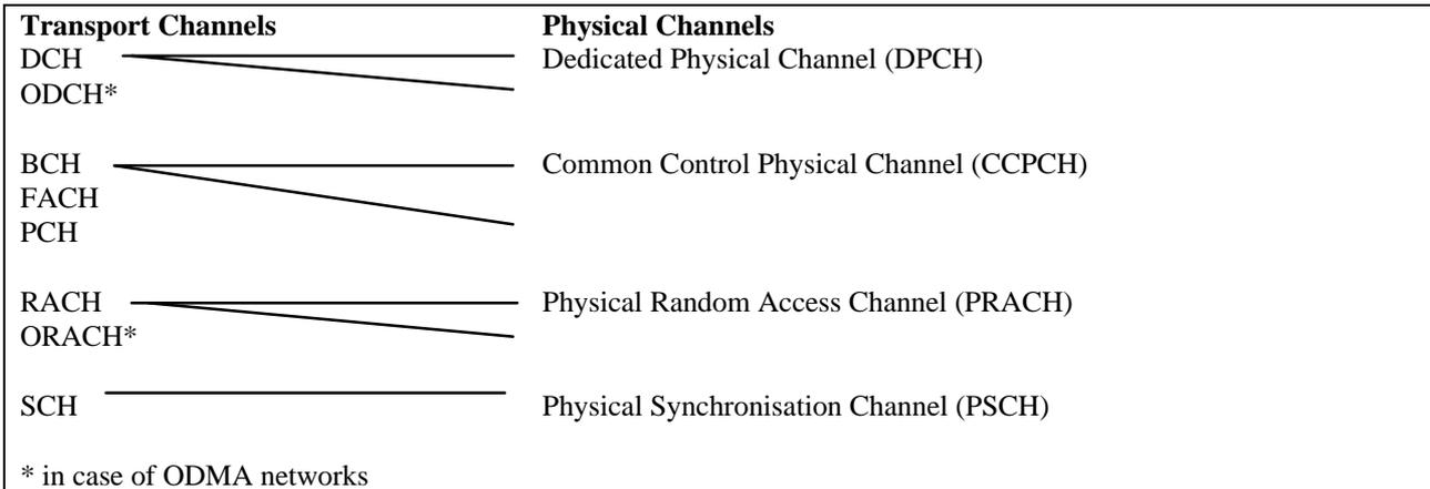
**Figure 11 Transport channel to physical channel mapping**
