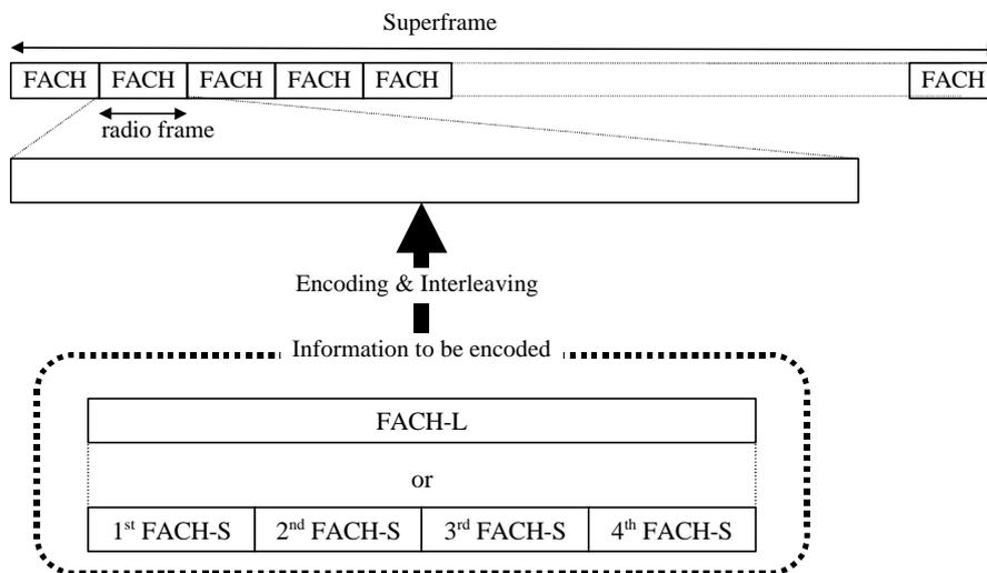
Fig. 3.2.1-7 FACH Mapping Method
