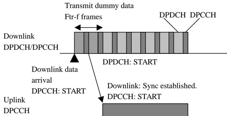
**Figure 6: Transmission resumption of downlink DPDCH**
