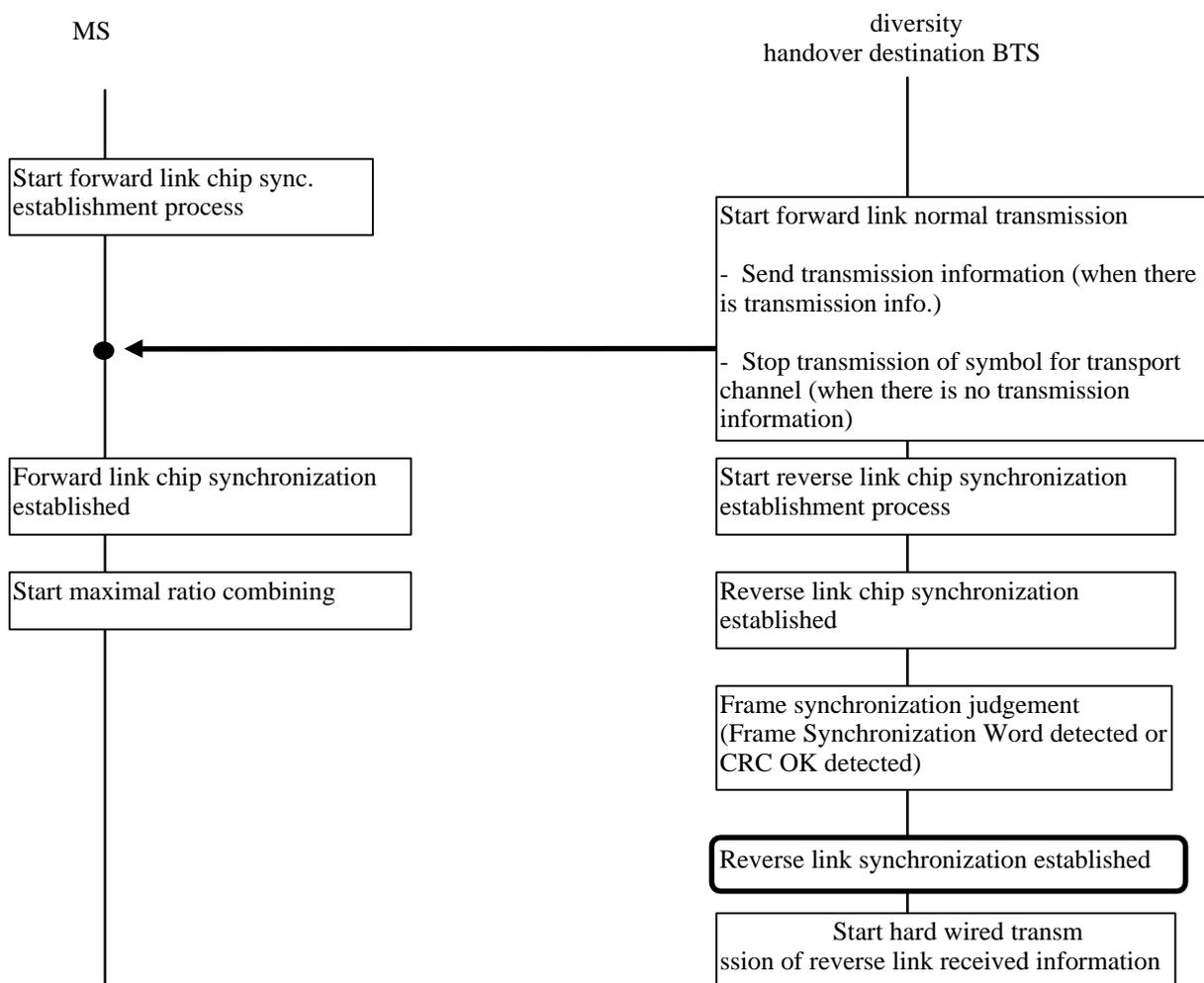
Fig. 3.2.6-4 Synchronization Establishment Flow Upon Intra/Inter-cell Diversity Handover
