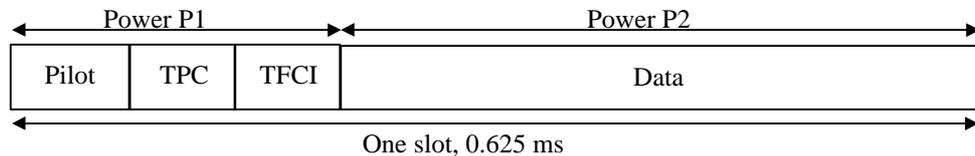
**Figure 3: Power setting of the downlink Dedicated Physical Channel**
