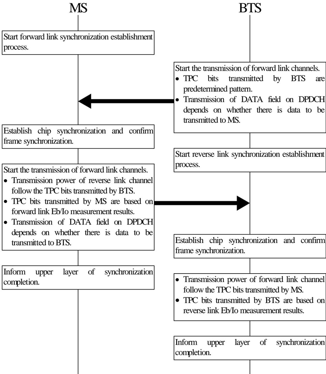
Fig.3.2.6-1 Synchronization Establishment Flow of Dedicated Channels
