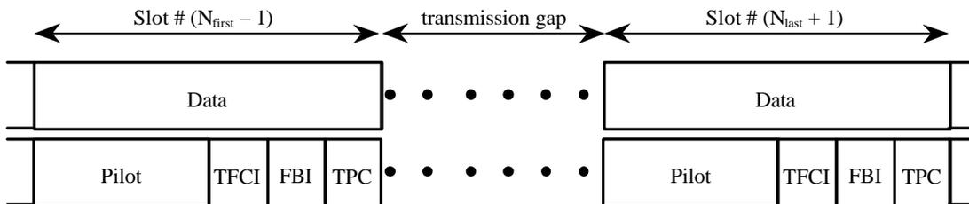
Figure 12: Frame structure in uplink compressed transmission
