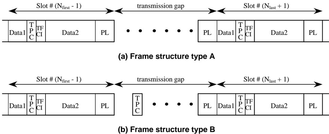
**Figure 13: Frame structure types in downlink compressed transmission**
