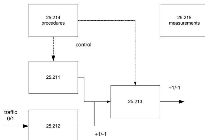
**Figure 1 - signal flow in FDD**
