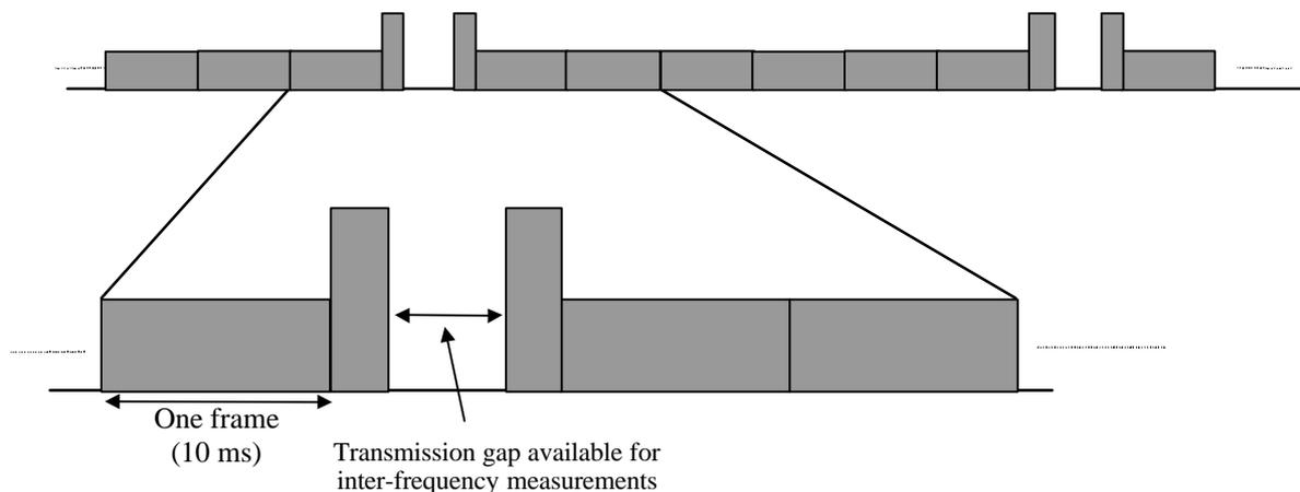
Figure 12: Compressed mode transmission
