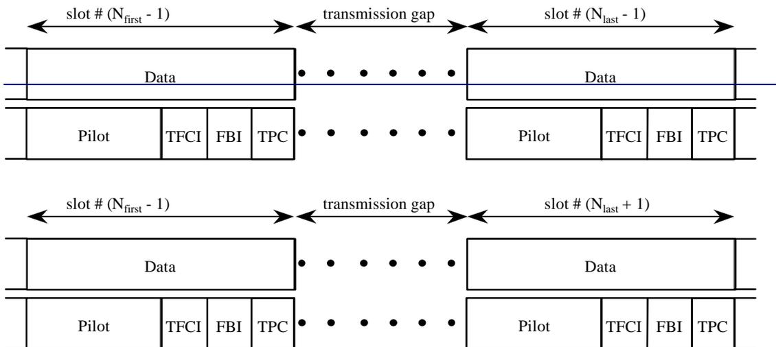
Figure 13: Frame structure in uplink compressed transmission
