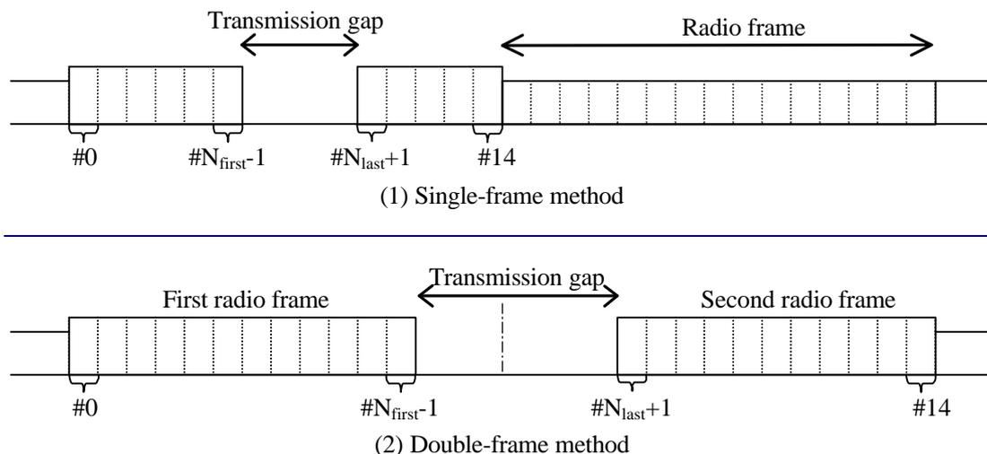
**Figure 15: Fixed transmission gap position**
