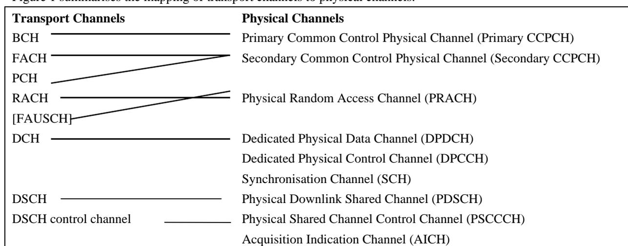
**Figure 1: Transport-channel to physical-channel mapping.**
