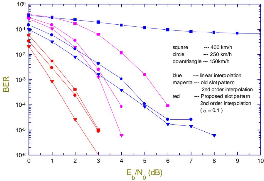
Fig 6. Receiver Performance of Different Velocity
