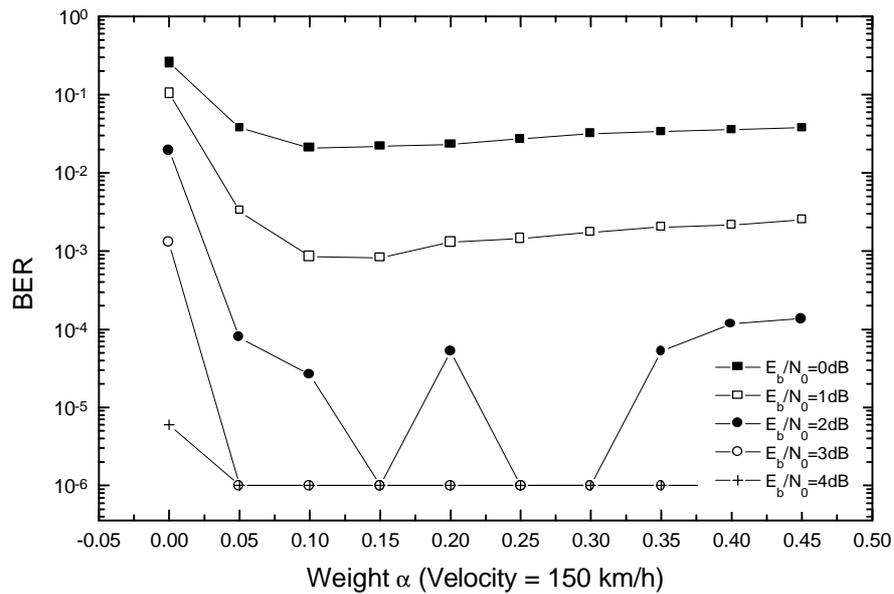
Fig3.Receiver Performance at Velocity of 150 km/h
