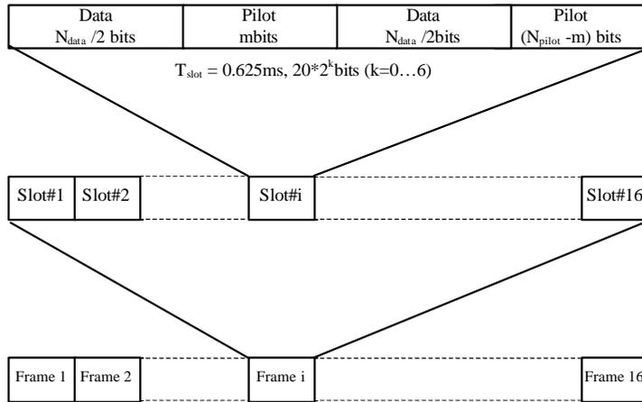
Fig. 2 Proposed Slot and Frame Structure
