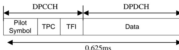
**Fig.1** Slot structure for forward link dedicated physical channel
