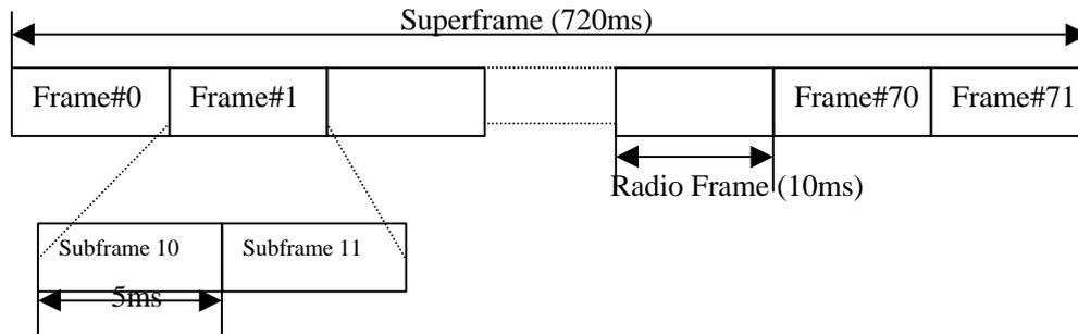
Figure 1. Frame structure
