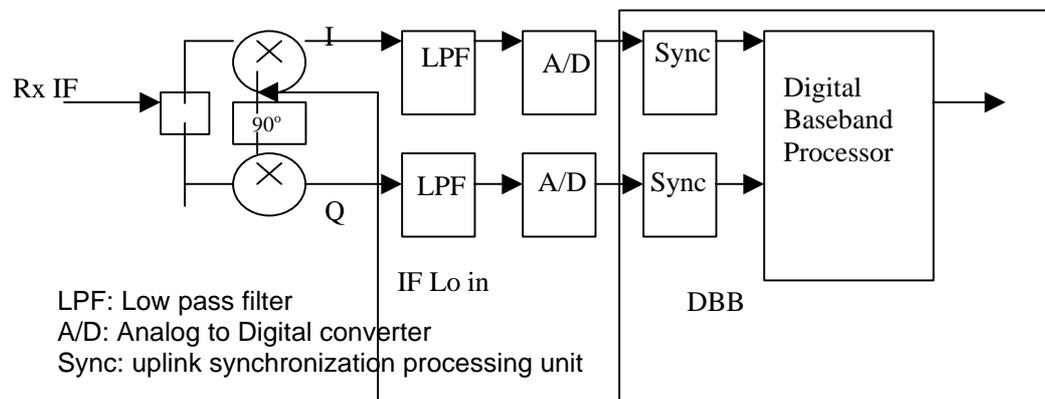
Figure 3. Example for DBB receiver used in synchronous CDMA and smart antenna system
