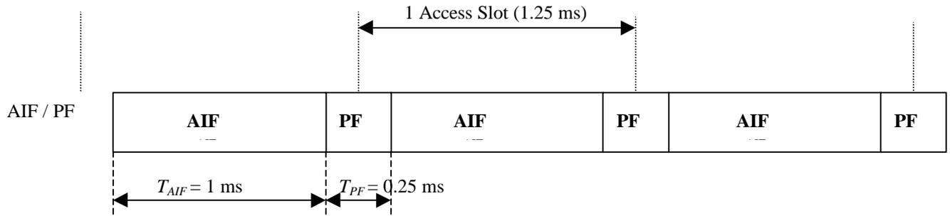
Figure 2 PF/AIF Multiplexing
