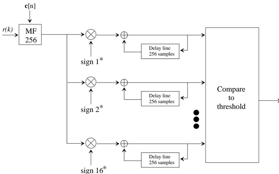
**Figure 1. Block diagram of the preamble detector using long codes.**
