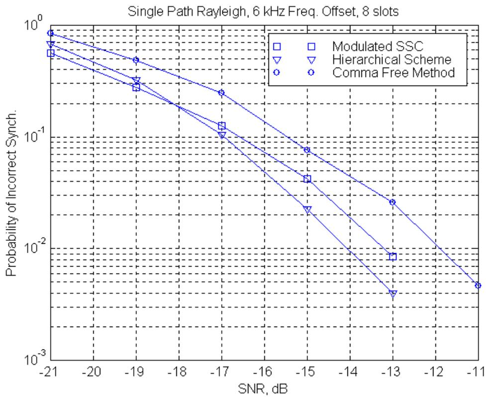
**Fig. 8: Probability of incorrect code group/frame timing synchronization in single Rayleigh fading, 8 slots integration is used.**
