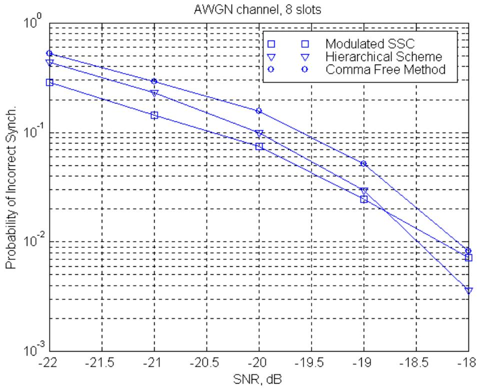
**Fig. 6: Probability of incorrect code group/frame timing synchronization in AWGN, 8 slots integration is used.**
