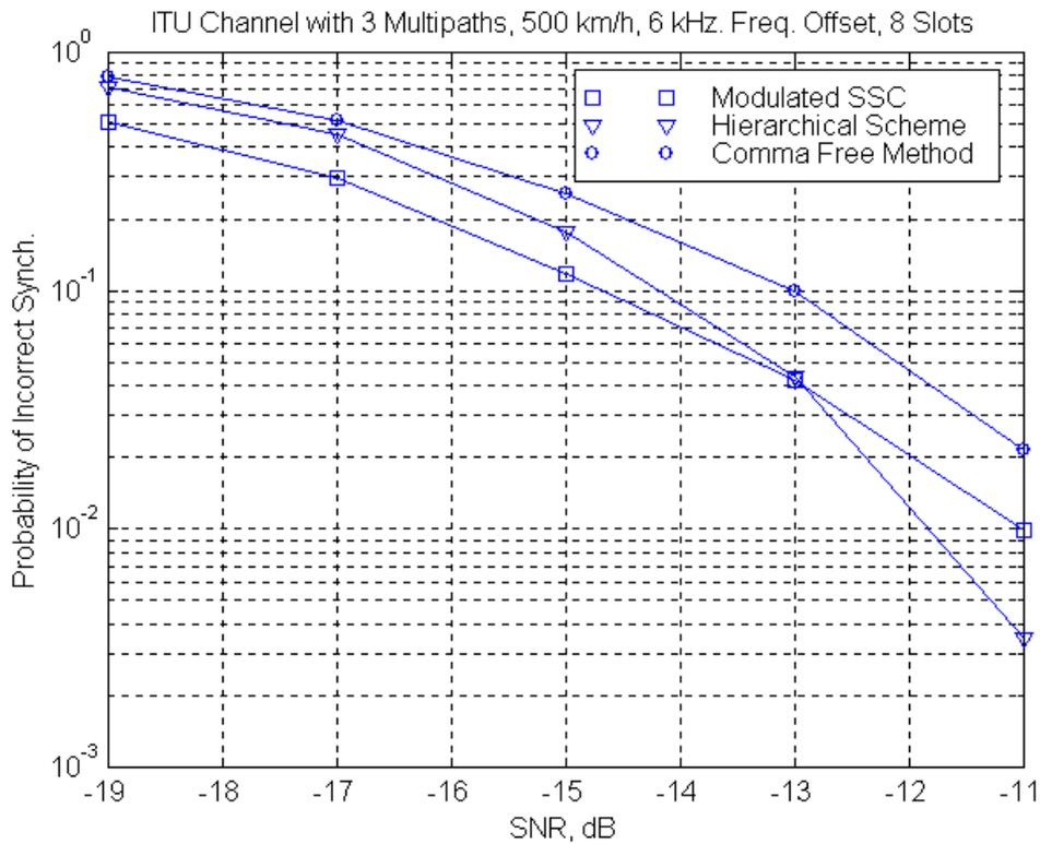
**Fig. 10: Probability of incorrect code group/frame timing synchronization in ITU channel with 3 multipaths, 500 km/h doppler, 6kHz Freq. error, 8 slot integration.**
