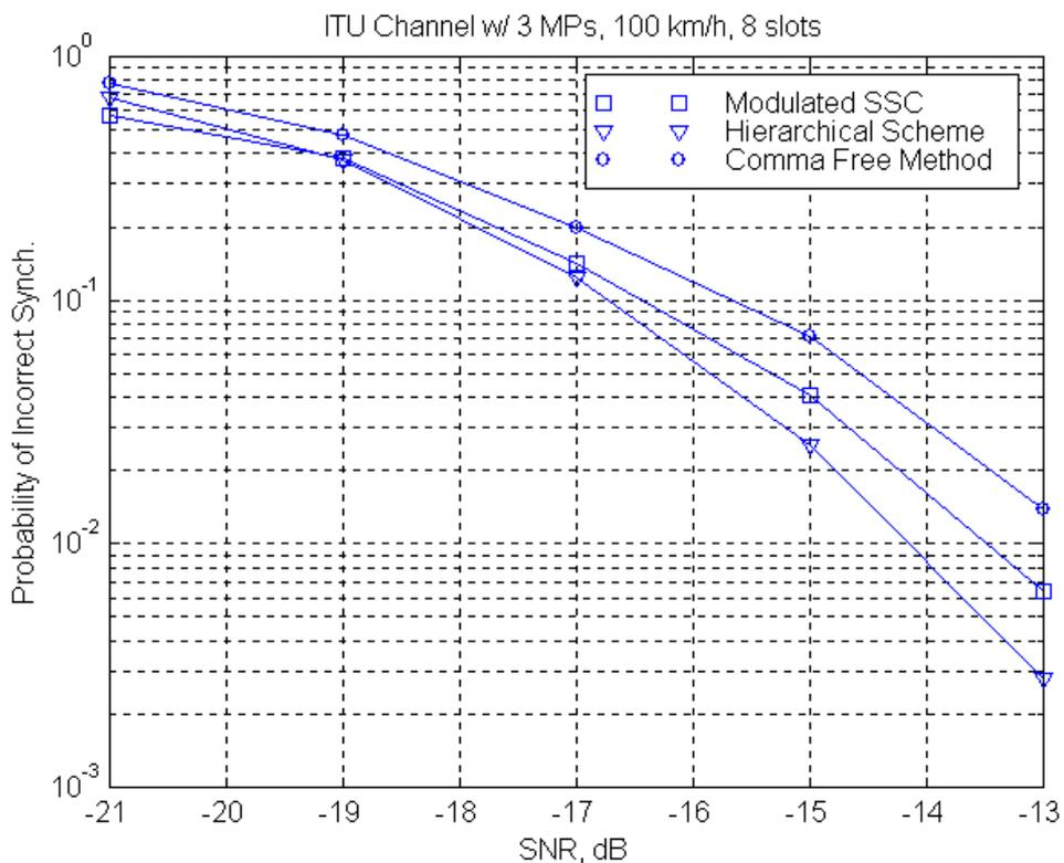
**Fig. 9: Probability of incorrect code group/frame timing synchronization in ITU channel with 3 multipaths (0, -6.9, -2.4 dB), 100 km/h doppler, 8 slot integration.**
