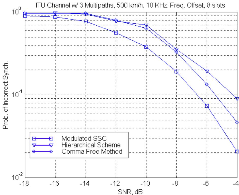
**Fig. 12: Probability of incorrect code group/frame timing synchronization in ITU Ch. with 3 multipaths, 500 km/h doppler, 10 kHz Freq. Offset, 8 slot integration.**
