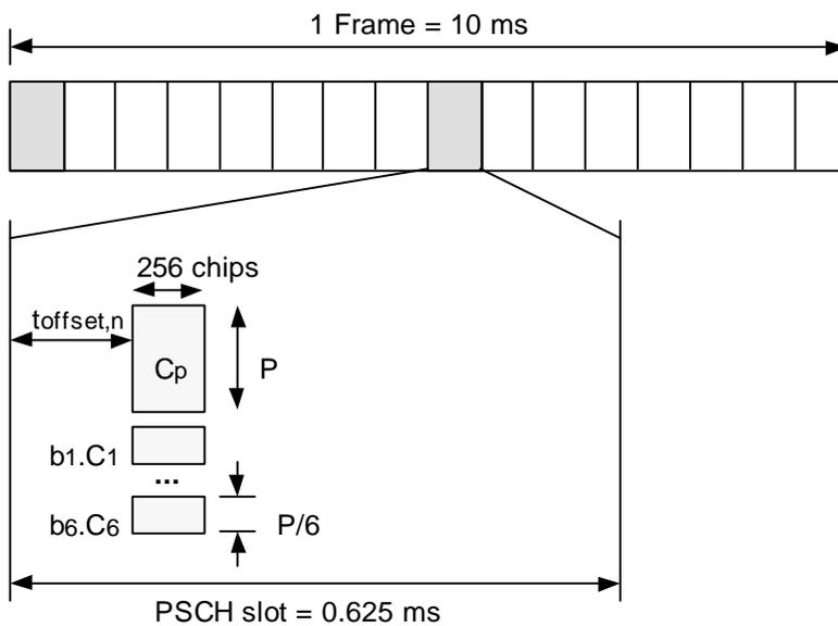
**Fig 1: The Physical Synchronization Channel (PSCH) Structure for the Proposed Scheme.**
