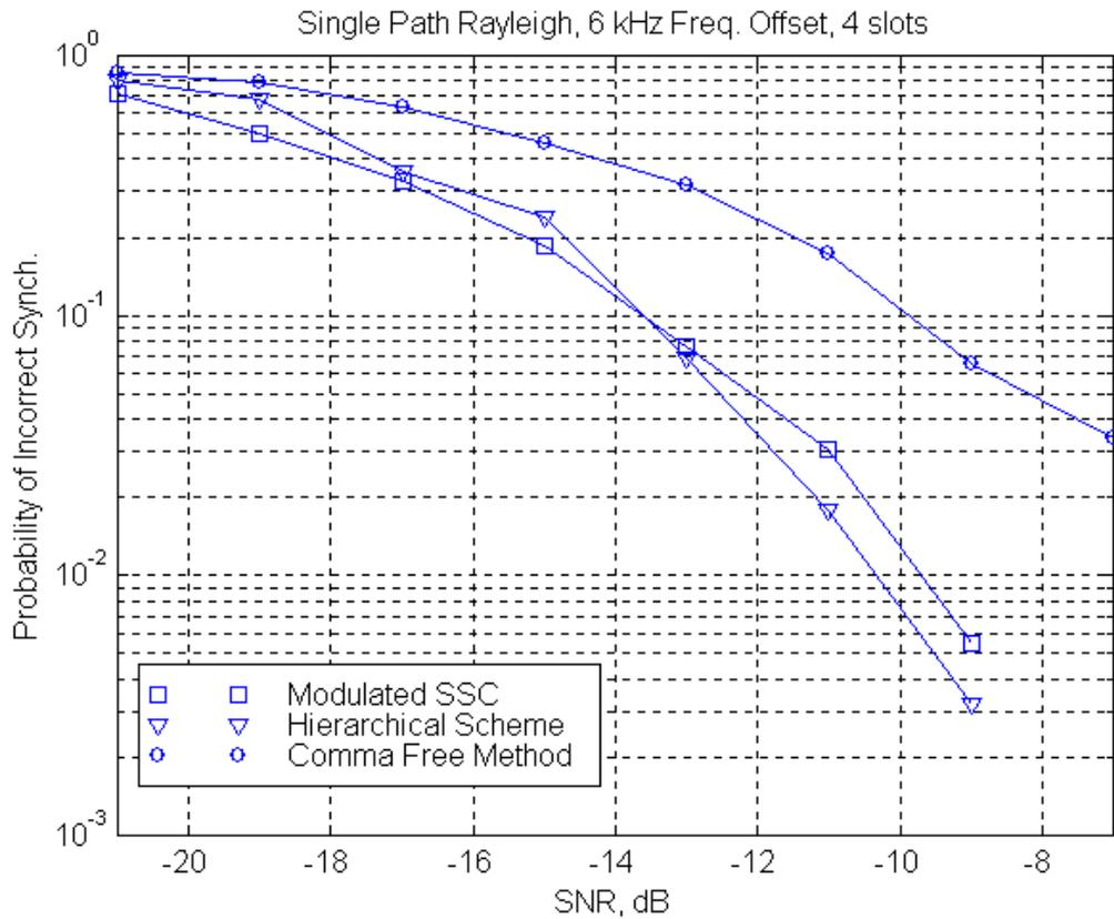
**Fig. 7: Probability of incorrect code group/frame timing synchronization in single Rayleigh fading, 6 kHz Freq. Error, 4 slots integration is used.**
