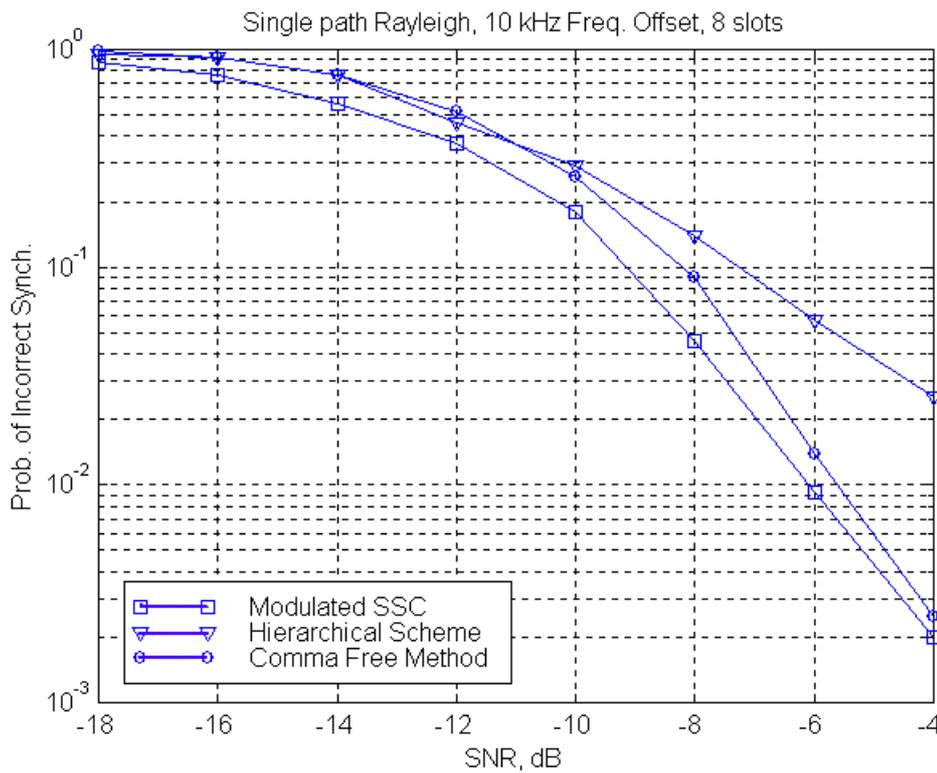
**Fig. 11: Probability of incorrect code group/frame timing synchronization in single Rayleigh fading, 10 kHz. freq. offset, 8 slots integration is used.**
