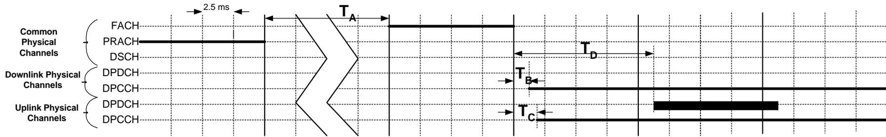
Figure 2 Rapid initialization of the DCH for transfer of uplink packet data.
