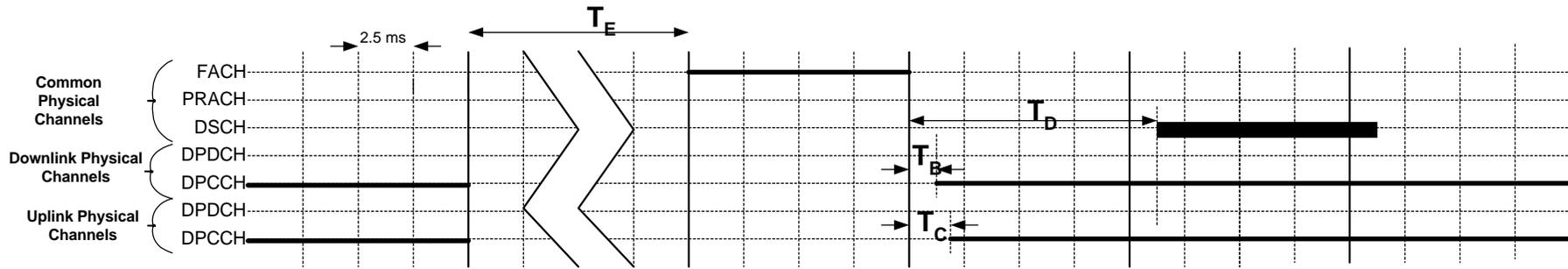
Figure 3 Resumption of the DCH for transmission of downlink packet data.
