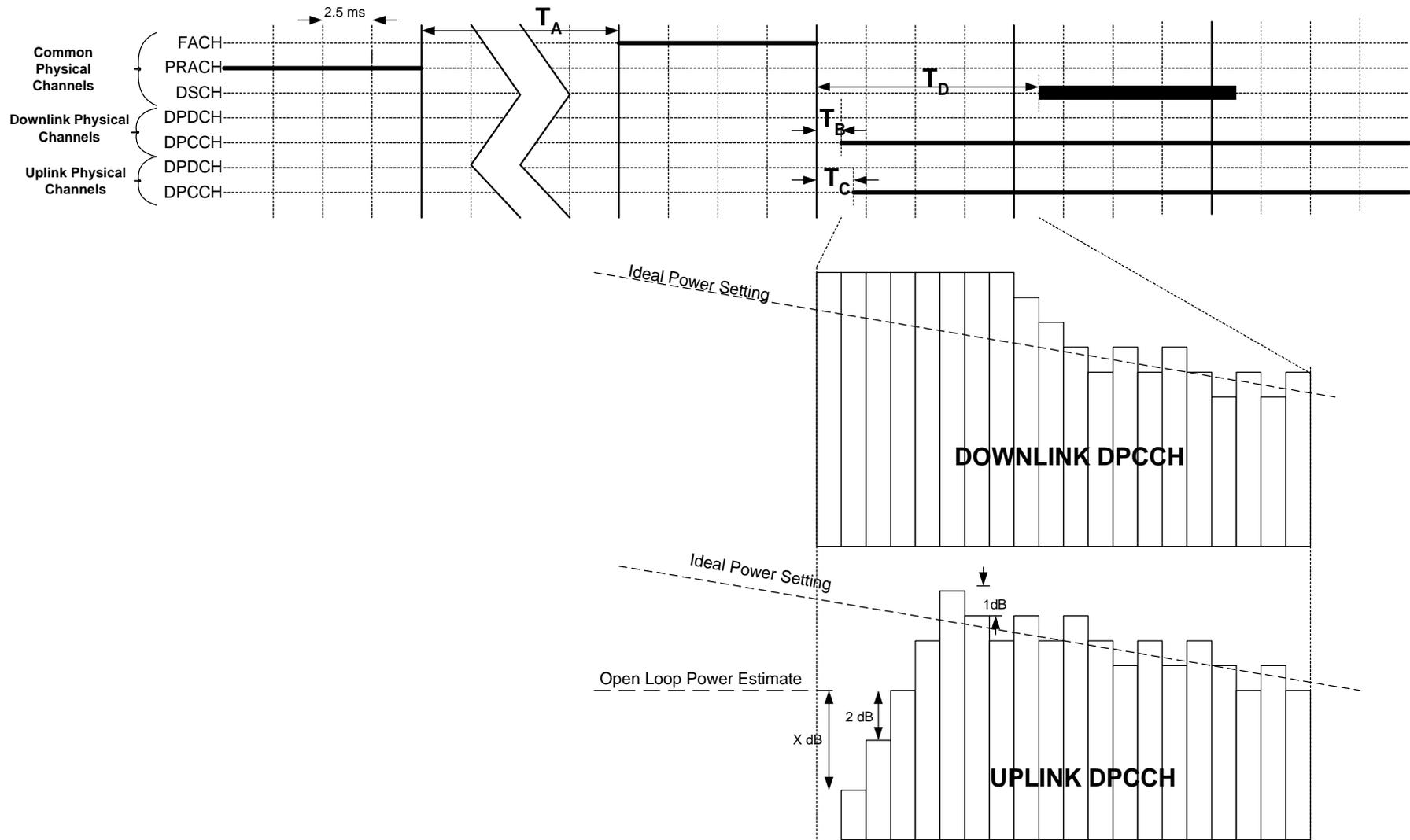
Figure 1 Rapid Initialization of DCH for packet data transfer over the DSCH.
