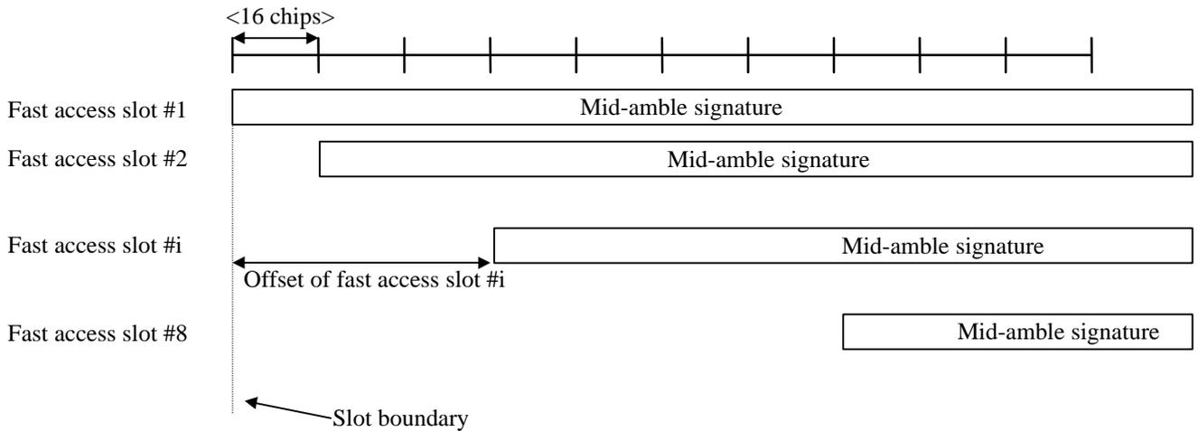
**Figure 4: PRACH Fast Access Bursts for FAUSCH (overlapping)**
