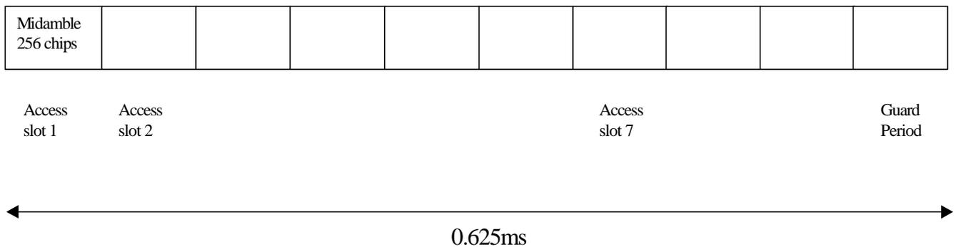
**Figure 3: PRACH Access Burst for FAUSCH (non-overlapping)**
