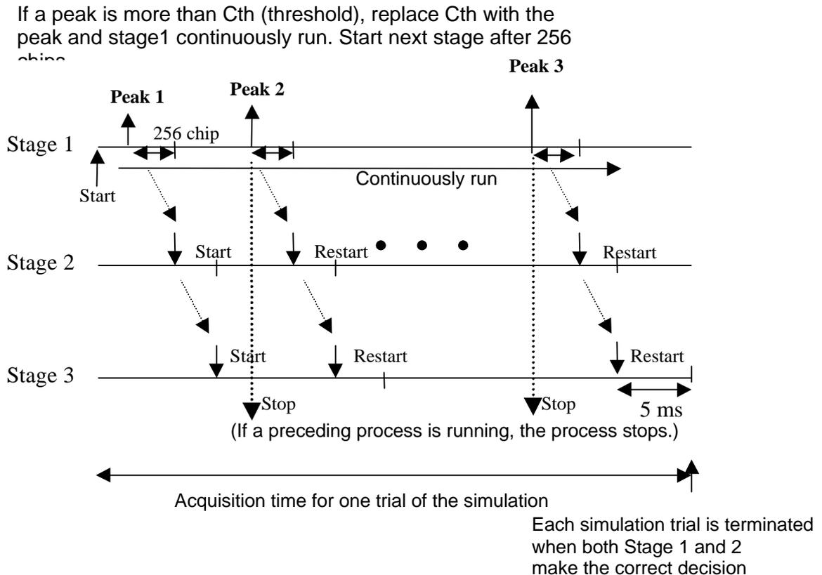
Fig. 2 Receiver operation for the synchronisation channel
