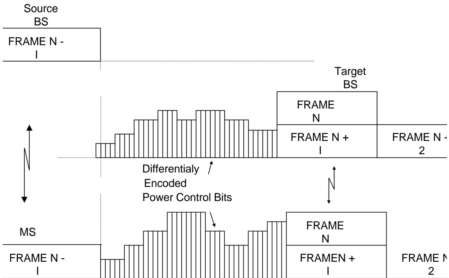
G 2. Timing Diagram of Handoff Process Using Code Multiplexing
