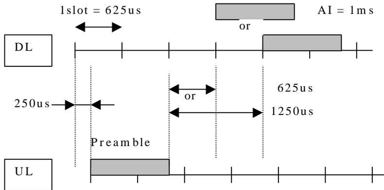
Fig.1 Value of Timing from Preamble to AI
