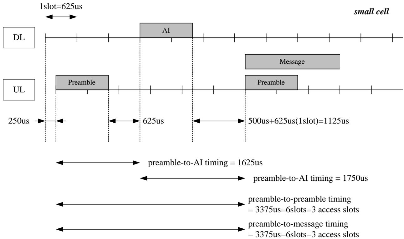
Fig.3 Timing of AICH transmission/reception (small cell)
