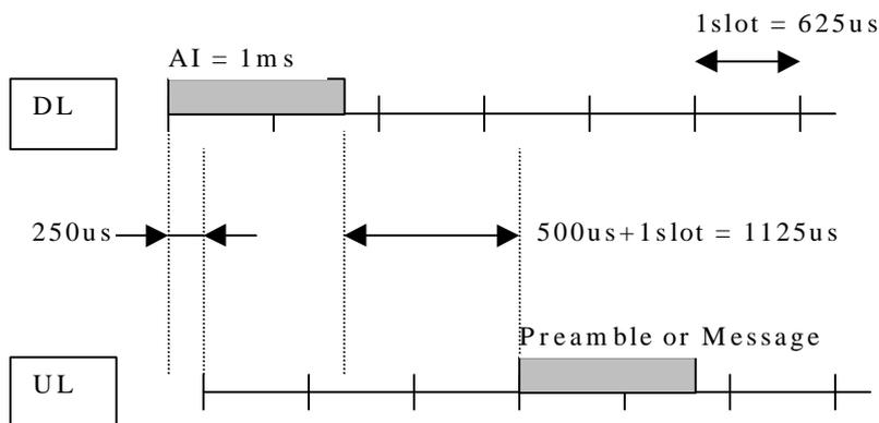
Fig.2 Minimum timing from AI to Preamble/Message
