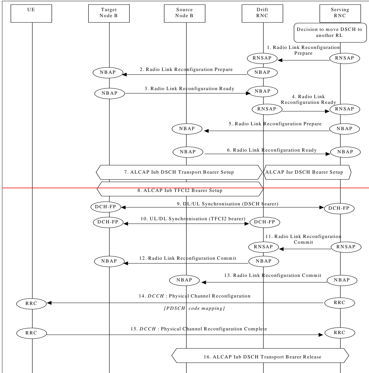
Figure 26a: DSCH mobility procedure in Soft Handover — (moving DSCH within the active set)
