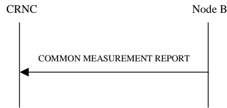
Figure 13: Common Measurement Reporting procedure, Successful Operation
