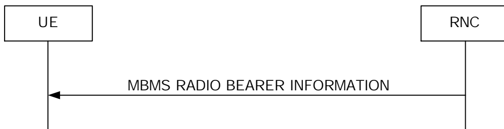
Figure 14: MBMS radio bearer information signalling flow
