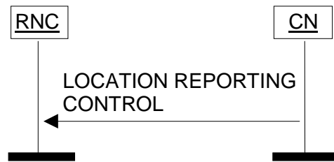
Figure 21: Location Reporting Control procedure. Successful operation.
