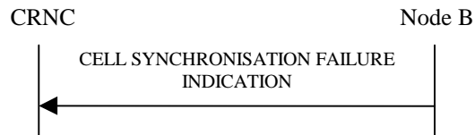
Figure 271 Cell Synchronisation Failure procedure, Successful Operation
