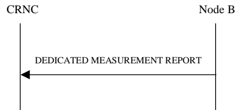
Figure 40: Dedicated Measurement Reporting procedure, Successful Operation
