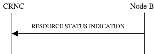
Figure 21: Resource Status Indication procedure, Successful Operation
