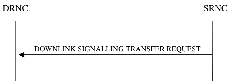
Figure 2: Downlink Signalling Transfer procedure, Successful Operation
