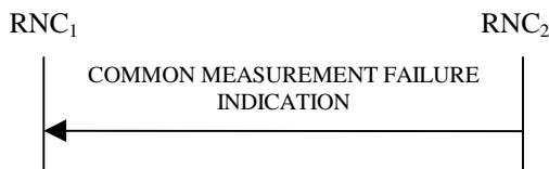
Figure 30E: Common Measurement Failure procedure, Successful Operation
