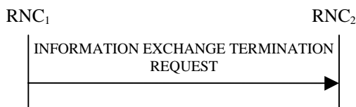
Figure 30I: Information Exchange Termination procedure, Successful Operation
