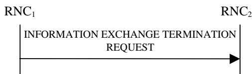
Figure 30I: Information Exchange Termination procedure, Successful Operation
