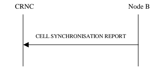
Figure 5 Cell Synchronisation Reporting procedure, Successful Operation
