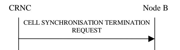
Figure 8 Cell Synchronisation Termination procedure, Successful Operation
